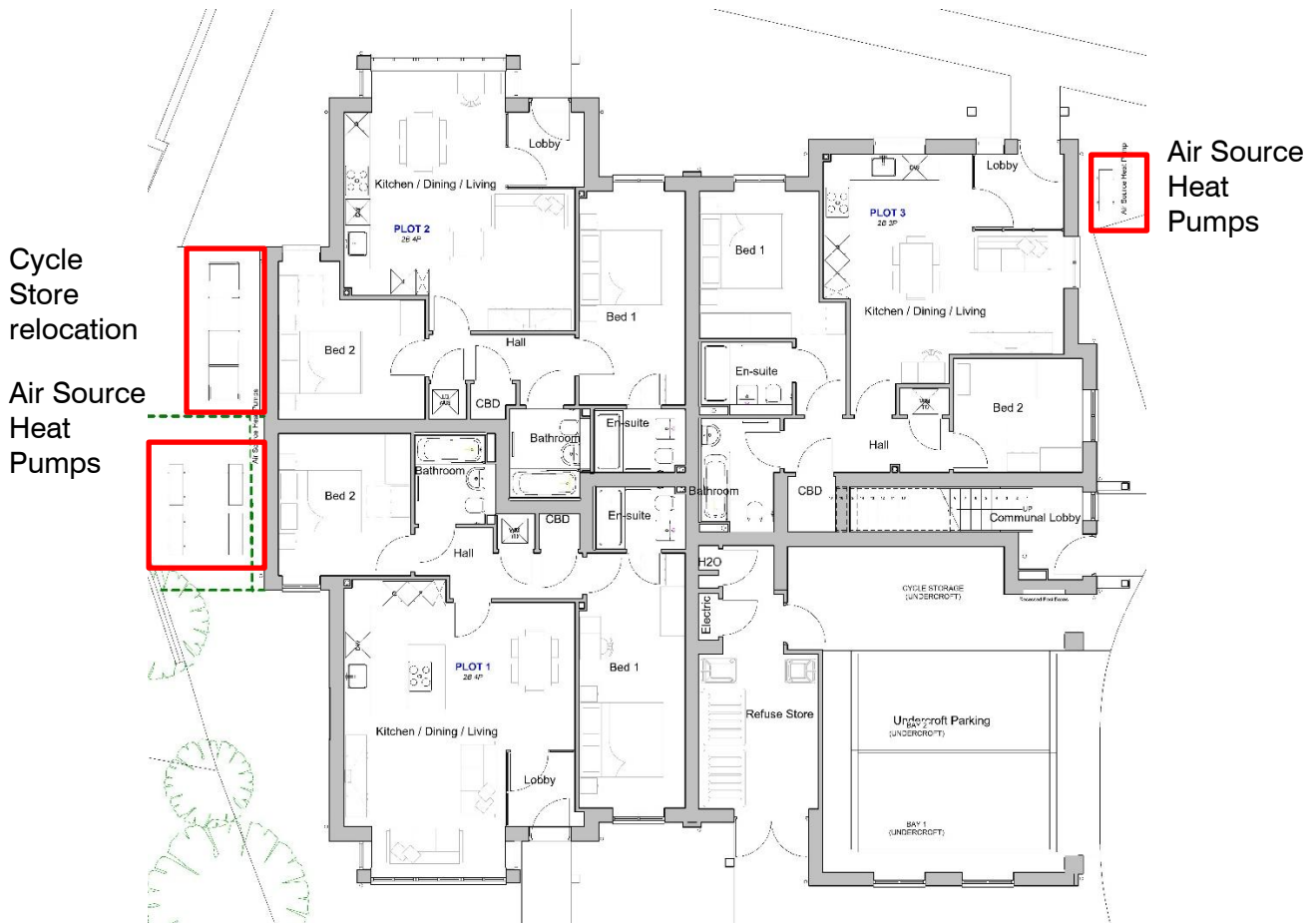
Proposed Ground Floor Plan- illustrating Air Source Heat Pump and Cycle Store Locations
