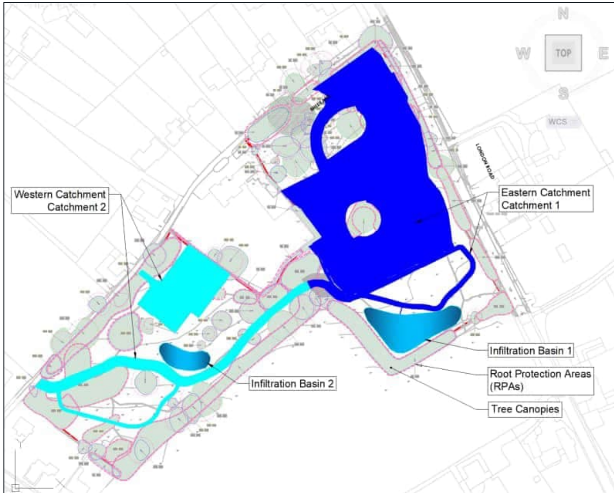
Figure 7-1 - Drainage Catchments and Infiltration Basins
