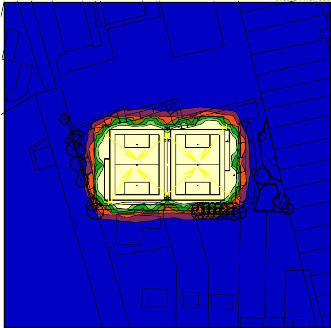
Figure 11 - Floodlighting Illuminance (Lux)
