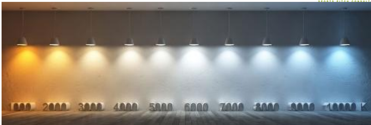
Figure 5 - Colour Temperature Illustration
