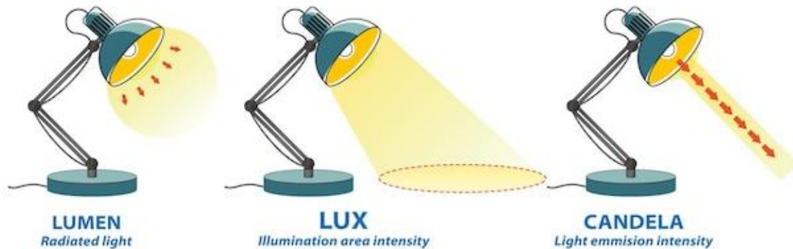
Figure 1 - Lumen, Lux and Candella Diagram
