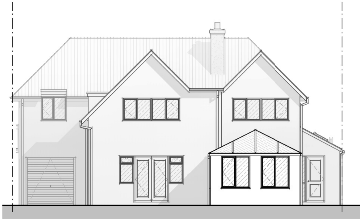
3 Rear Elevation - Existing 1 : 100 @A3
