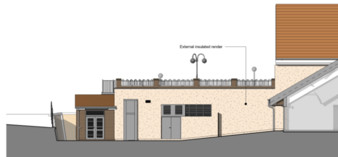
Plant Room South Elevation - Proposed
