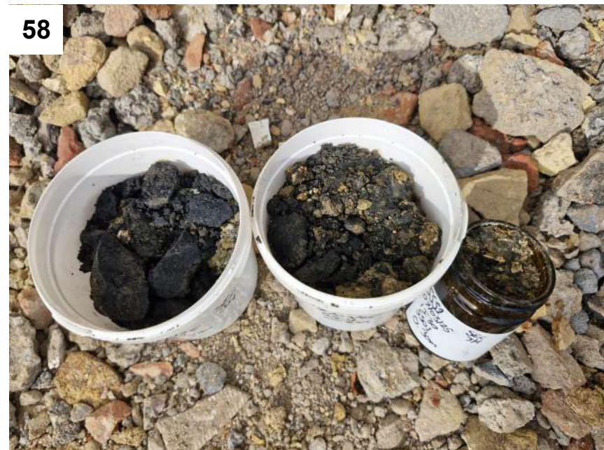
Photos 55 to 58 — View of the hydrocarbon stained material identified within the foundation trench between flats 1 and 2 with samples from that area SS01.
