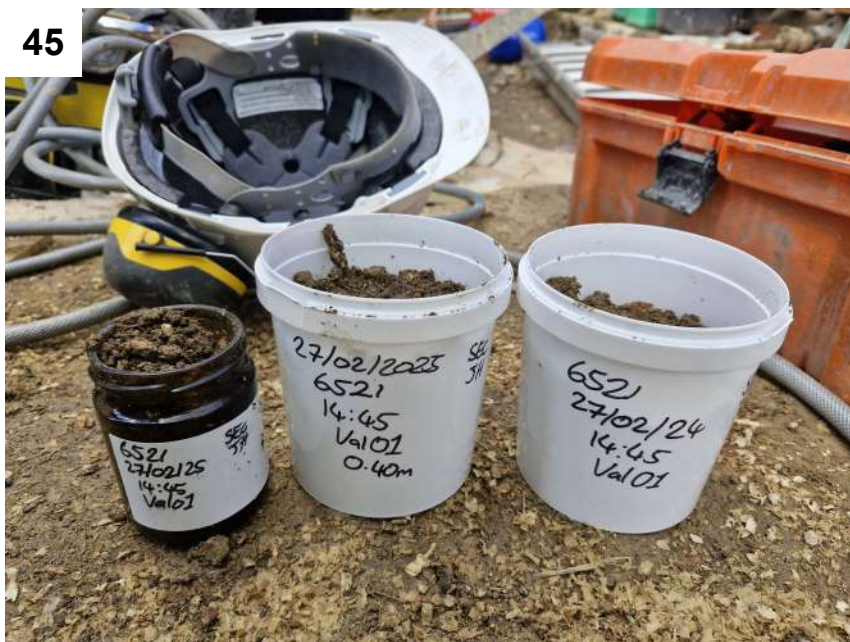
Photos 43 to 46 — View of the infilled soakaway feature identified to the western side of the site, the infill material and associated sampling - Val01.
