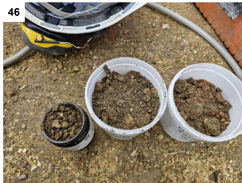
Photos 43 to 46 — View of the infilled soakaway feature identified to the western side of the site, the infill material and associated sampling - Val01.
