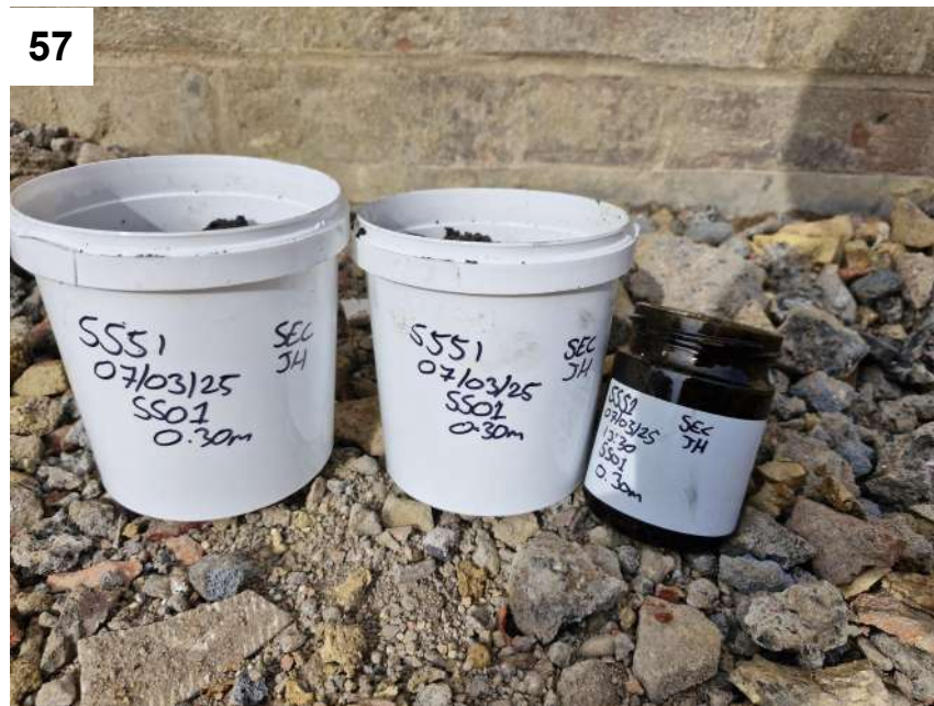
Photos 55 to 58 — View of the hydrocarbon stained material identified within the foundation trench between flats 1 and 2 with samples from that area SS01.
