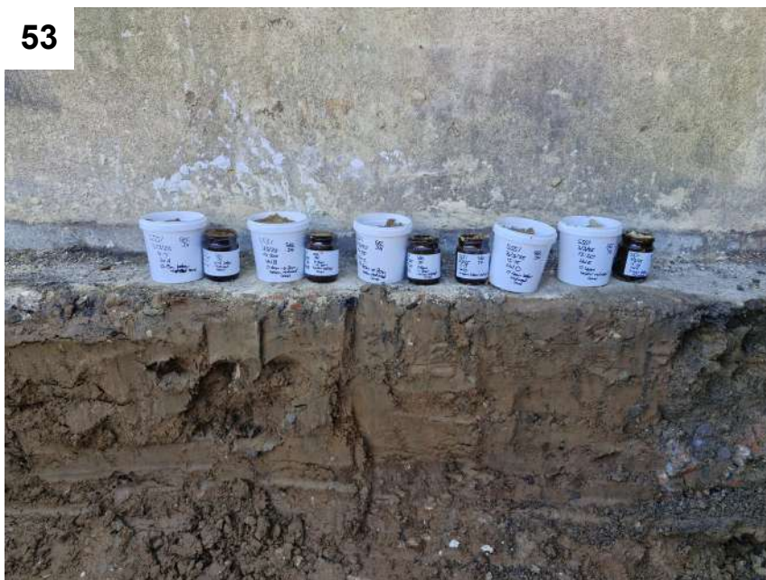
Photos 51 to 54 — View of the validation samples collected from the remedial excavation in the south west corner of the site
