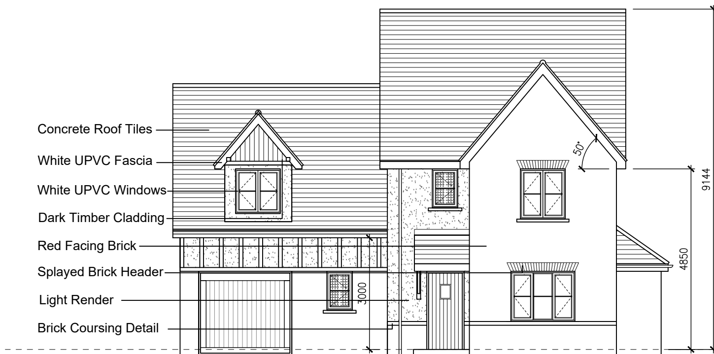
FRONT ELEVATION TYPE C2 PLOT 9
