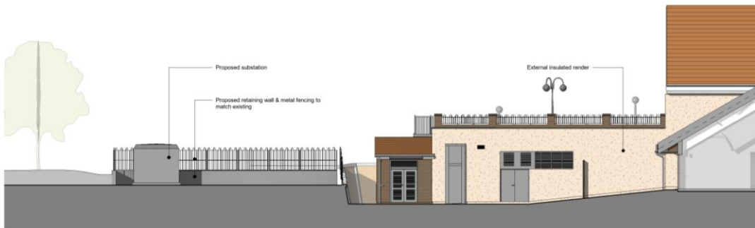
Plant Room South Elevation - Proposed
