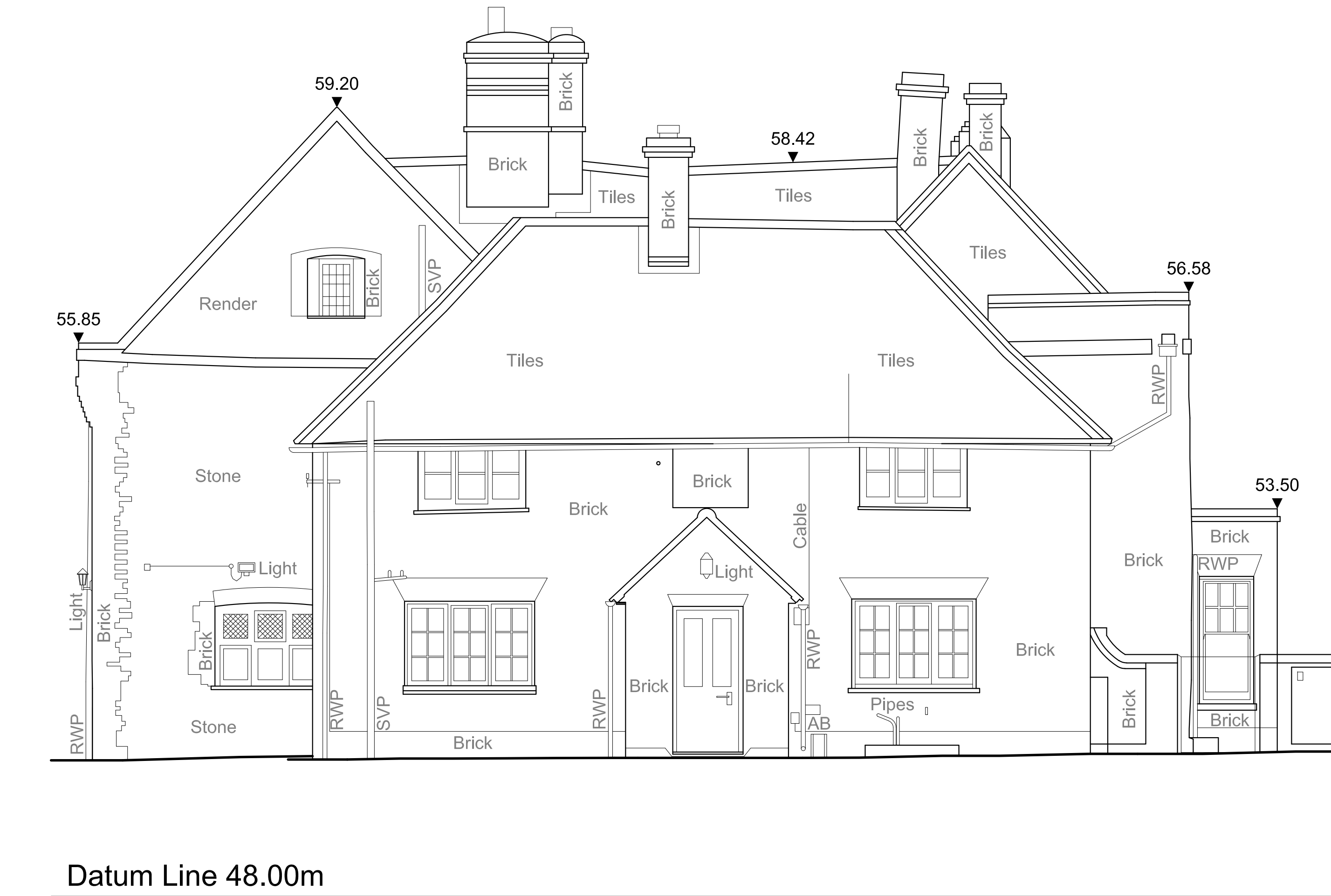
Elevation 4 (LH Side / West)
