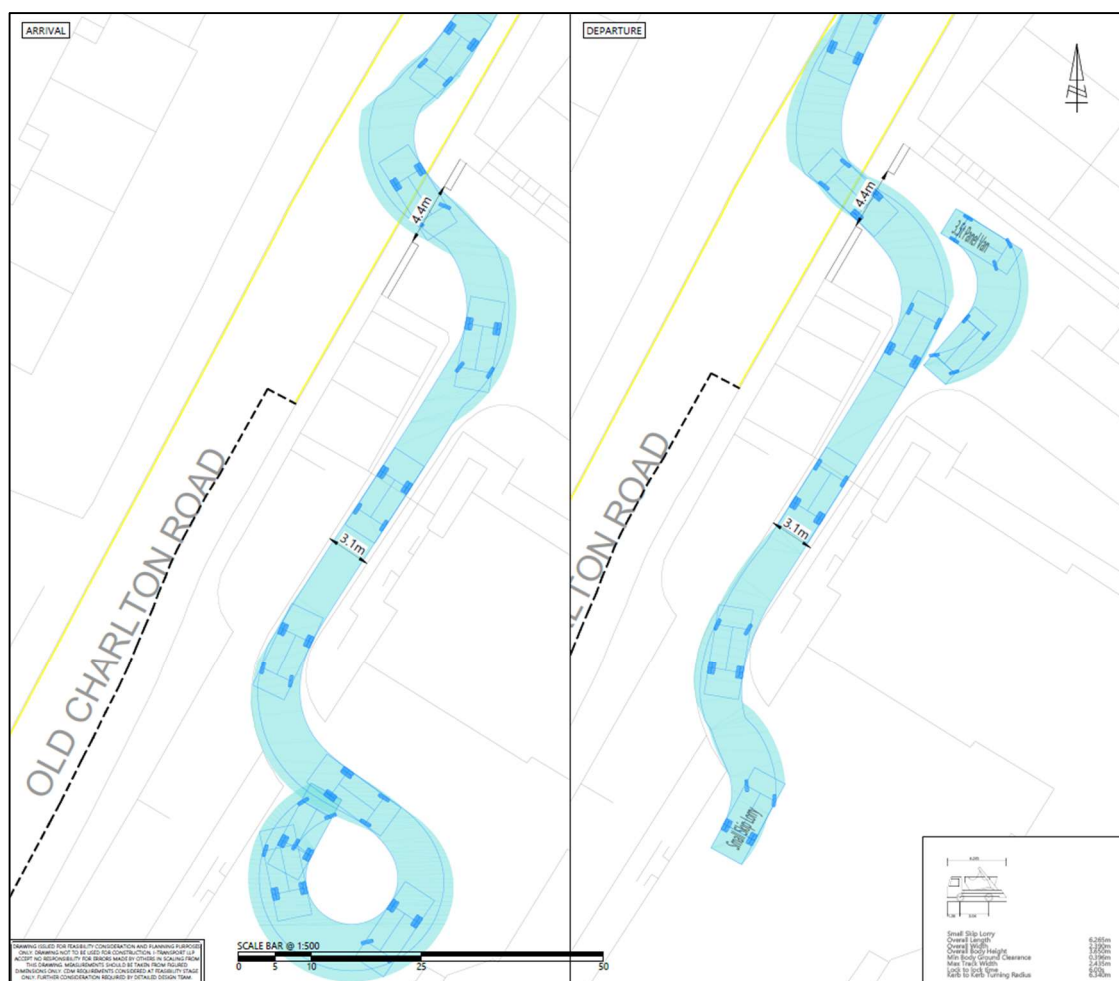
Figure 3.3 LGV/Small Skip Lorry Access
