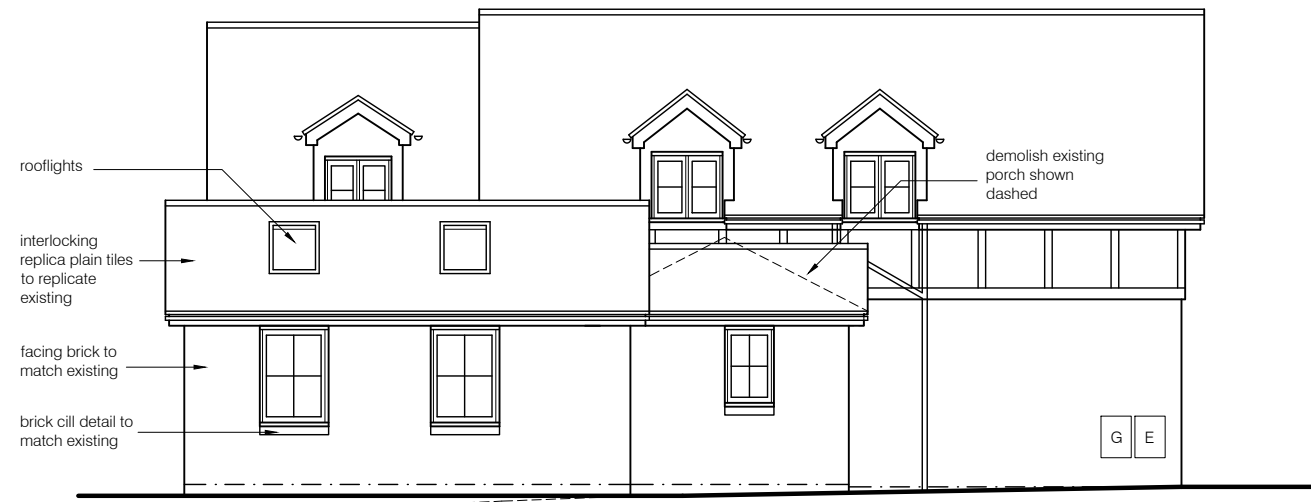
Side Elevation (north facing)
