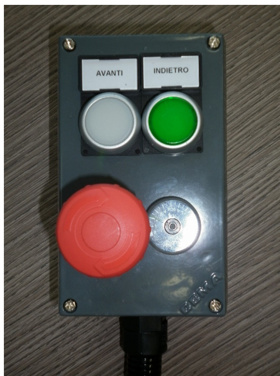
Picture 4 – Operating panel
