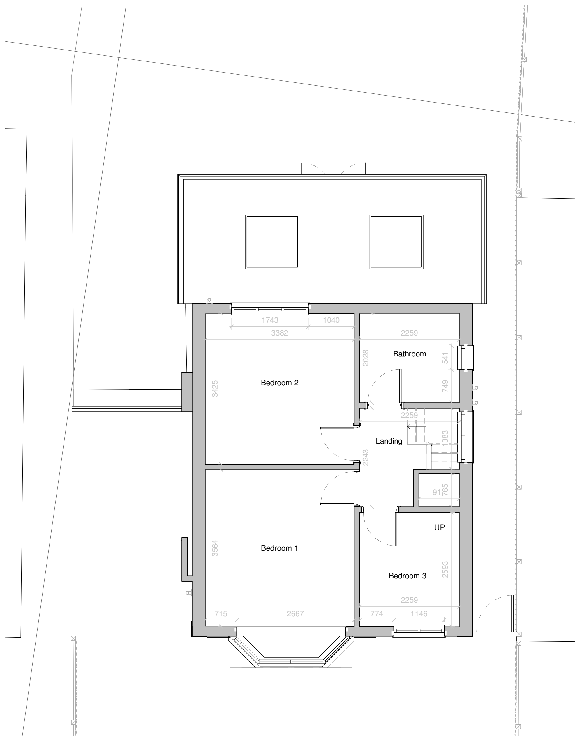
4 First Floor - As Existing 1 : 50
