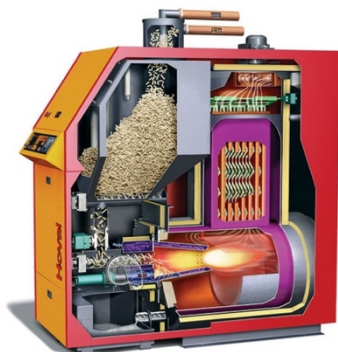
Figure 4: Biomass Boiler diagram
