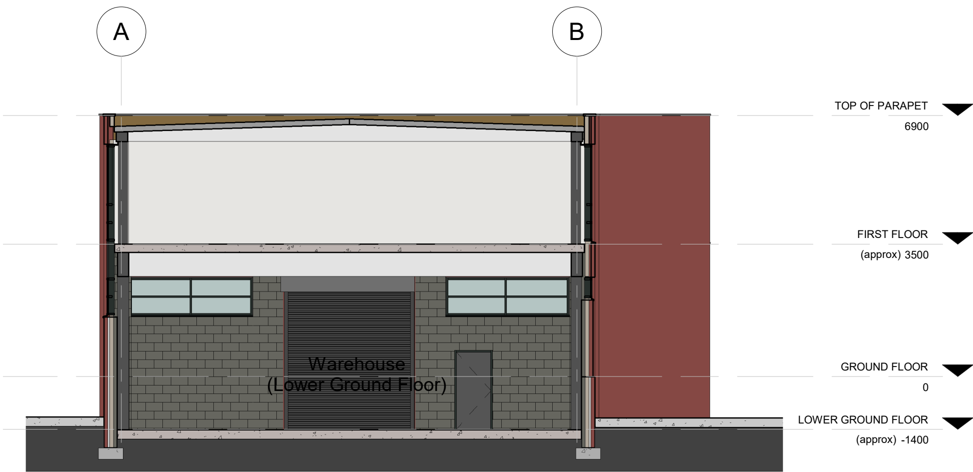
3 | Section 3 As Proposed (Planning) 1 : 100 | PL 06
