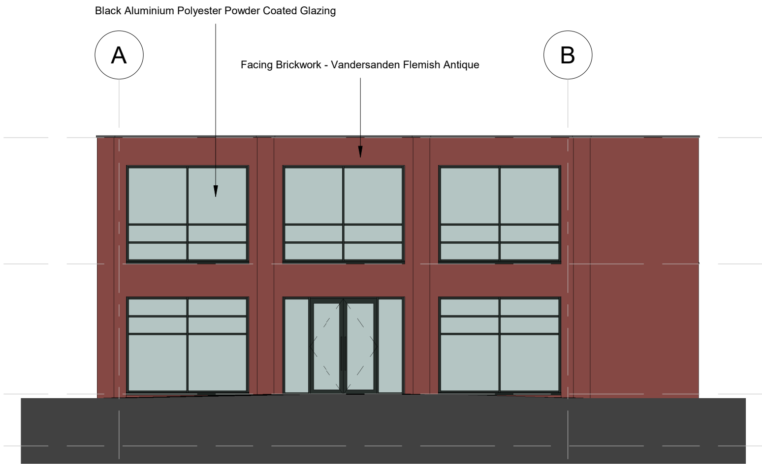
2 | End Elevation As Proposed (Ground Floor Level) (Planning)
