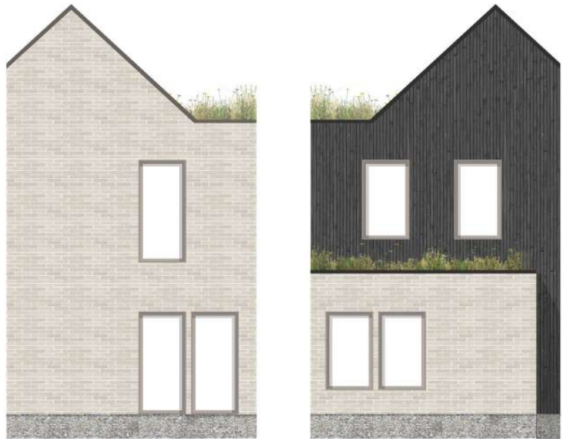
Option 4 Front - Polycor bricks with flint plinth Rear - Flint plinth with black stained timber cladding and Polycor bricks to ground floor protrusions
