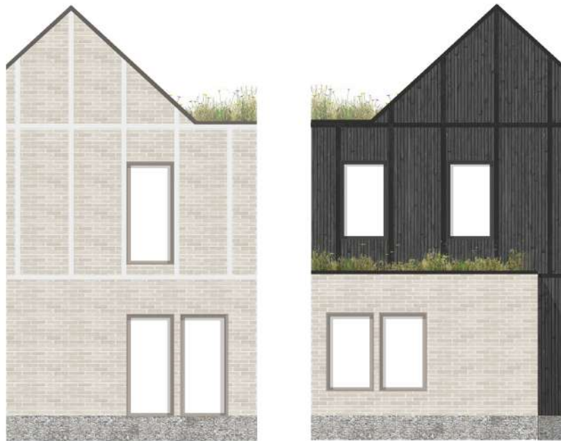
Option 6 Front - Flint plinth and Polycor brick with whitewashed timber frame exposed at first floor Rear - Black stained timber cladding and exposed timber frame to first floor with Polycor bricks to ground floor protrusions
