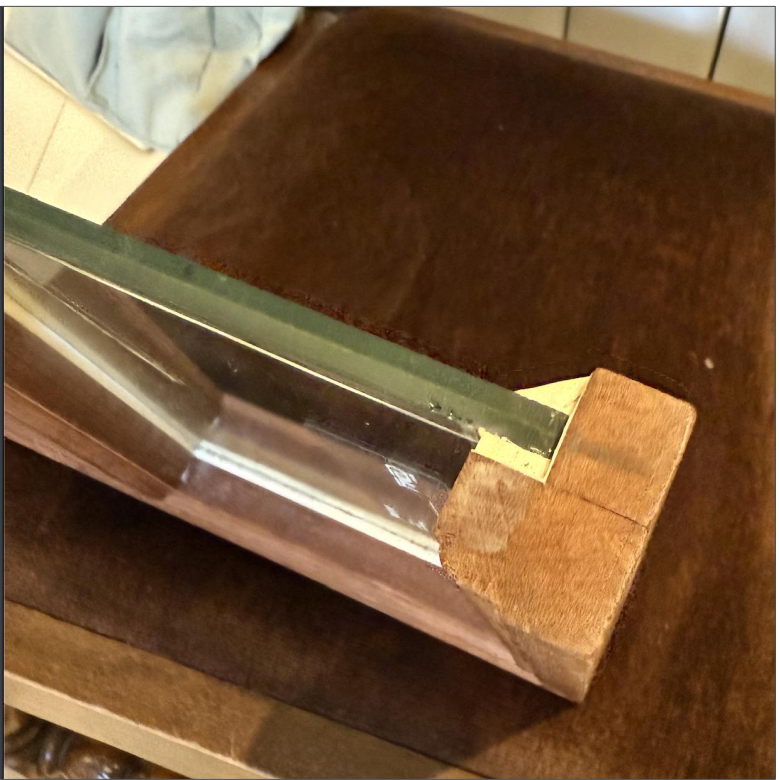
Above: Glazing upgrade mock up
