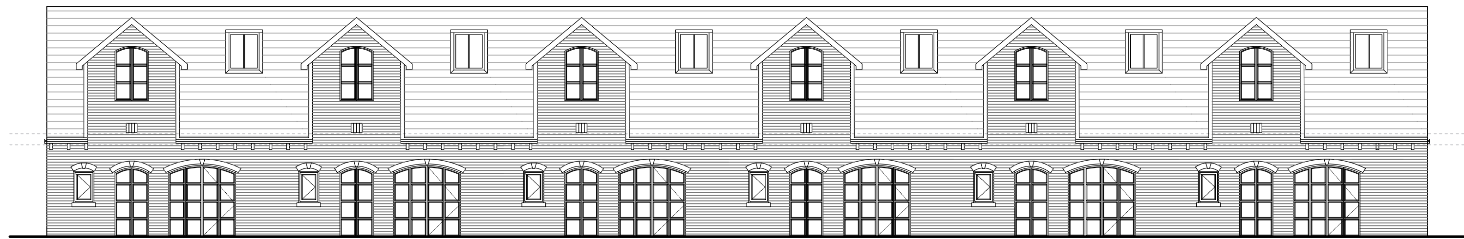
PROPOSED REAR ELEVATIONS - NORTH/EAST - UNITS 9 TO 14
