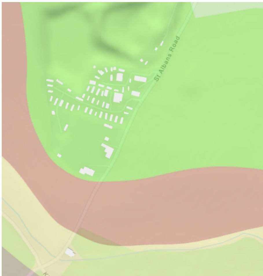
Figure 1 – Extract from British Geological Survey showing the application site as falling within the Lewes Nodular Chalk Formation
