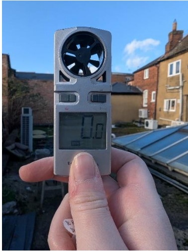
Figure 4 Onsite wind measurement
