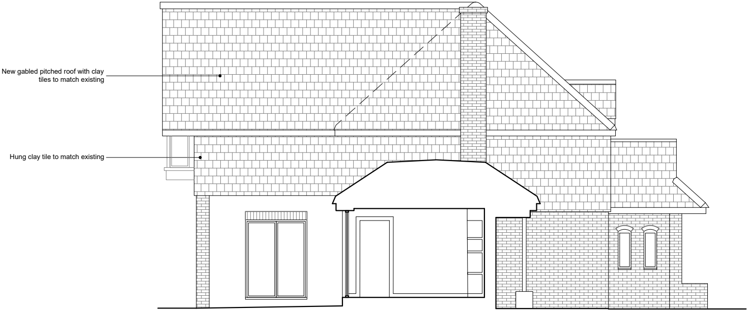
Side (East) Elevation
