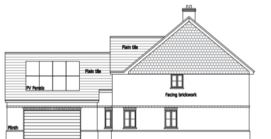
Side Elevation Solar Panels on Plot 4 only
