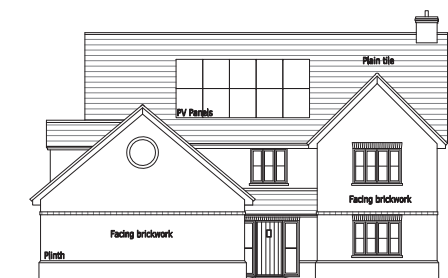
Front Elevation Solar Panels on Plot 5 ONLY
