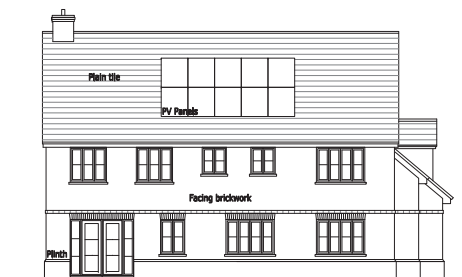
Rear Elevation Solar Panels on Plot 1 ONLY
