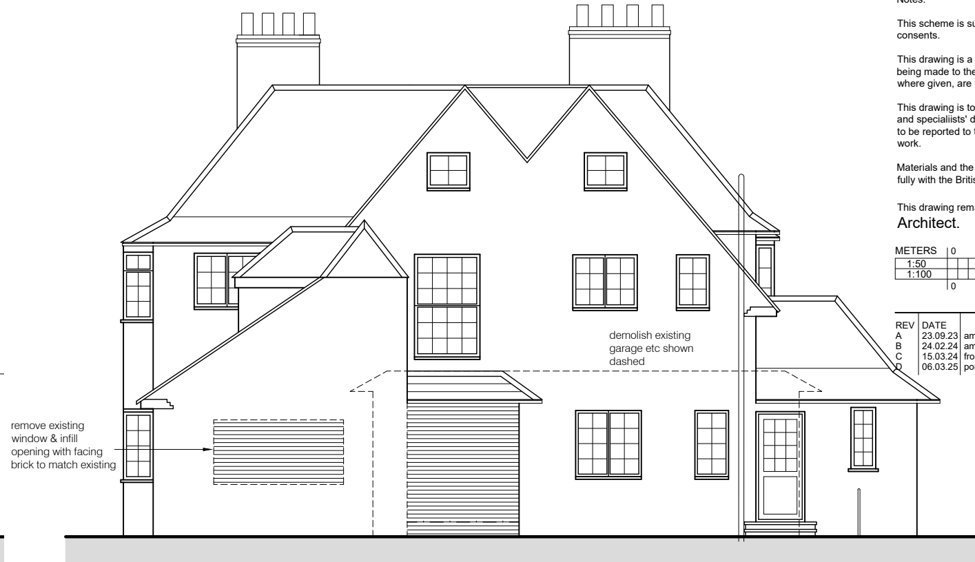
Side Elevation (south east facing)
