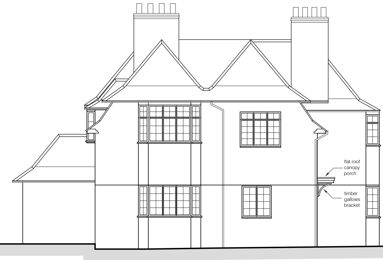
Side Elevation (north west facing)
