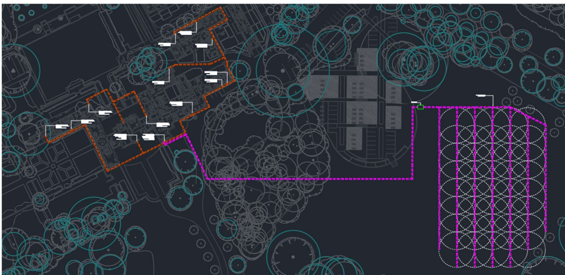
62No. boreholes and GSHP Manifold adjacent to Car Park
