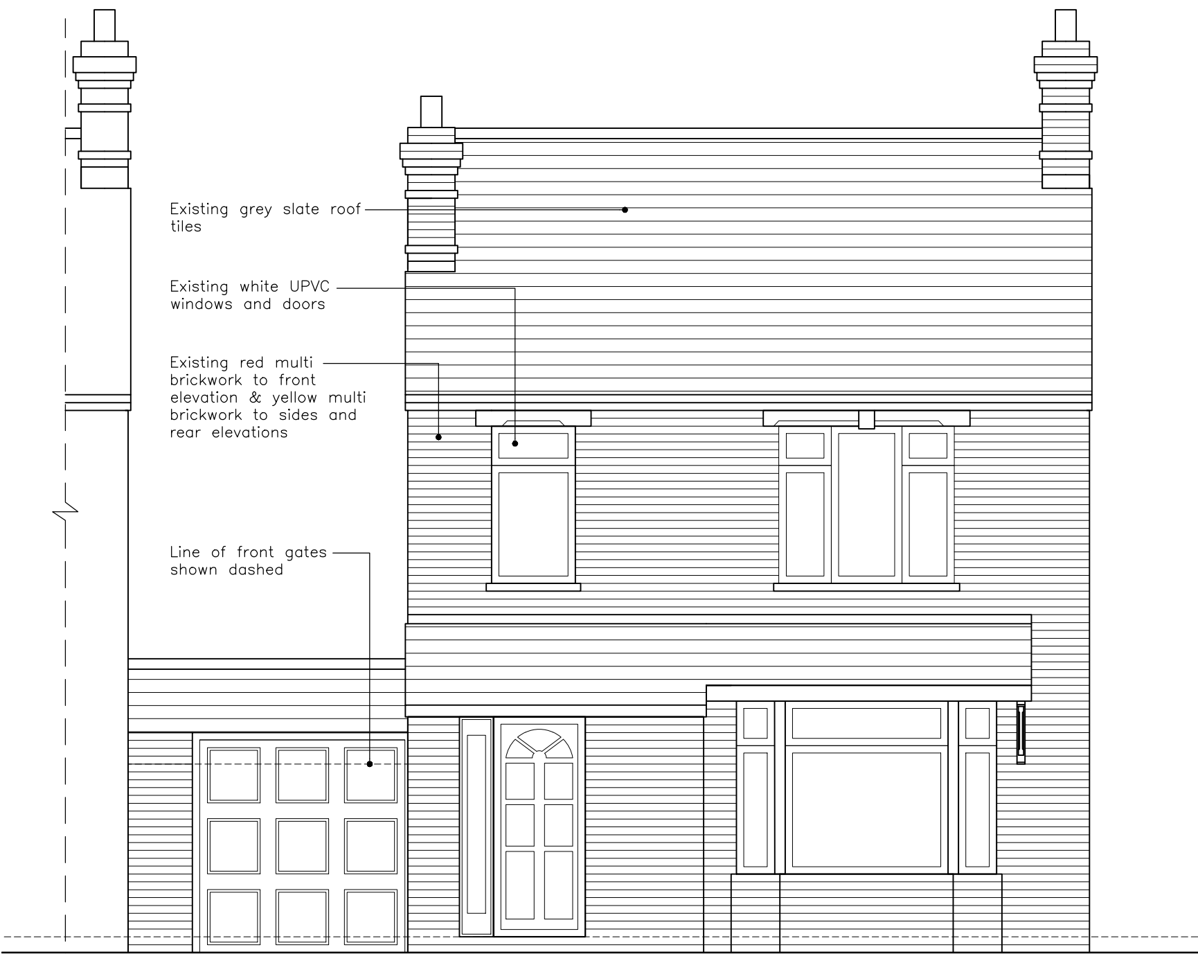
EXISTING FRONT ELEVATION 1: 50@A1
