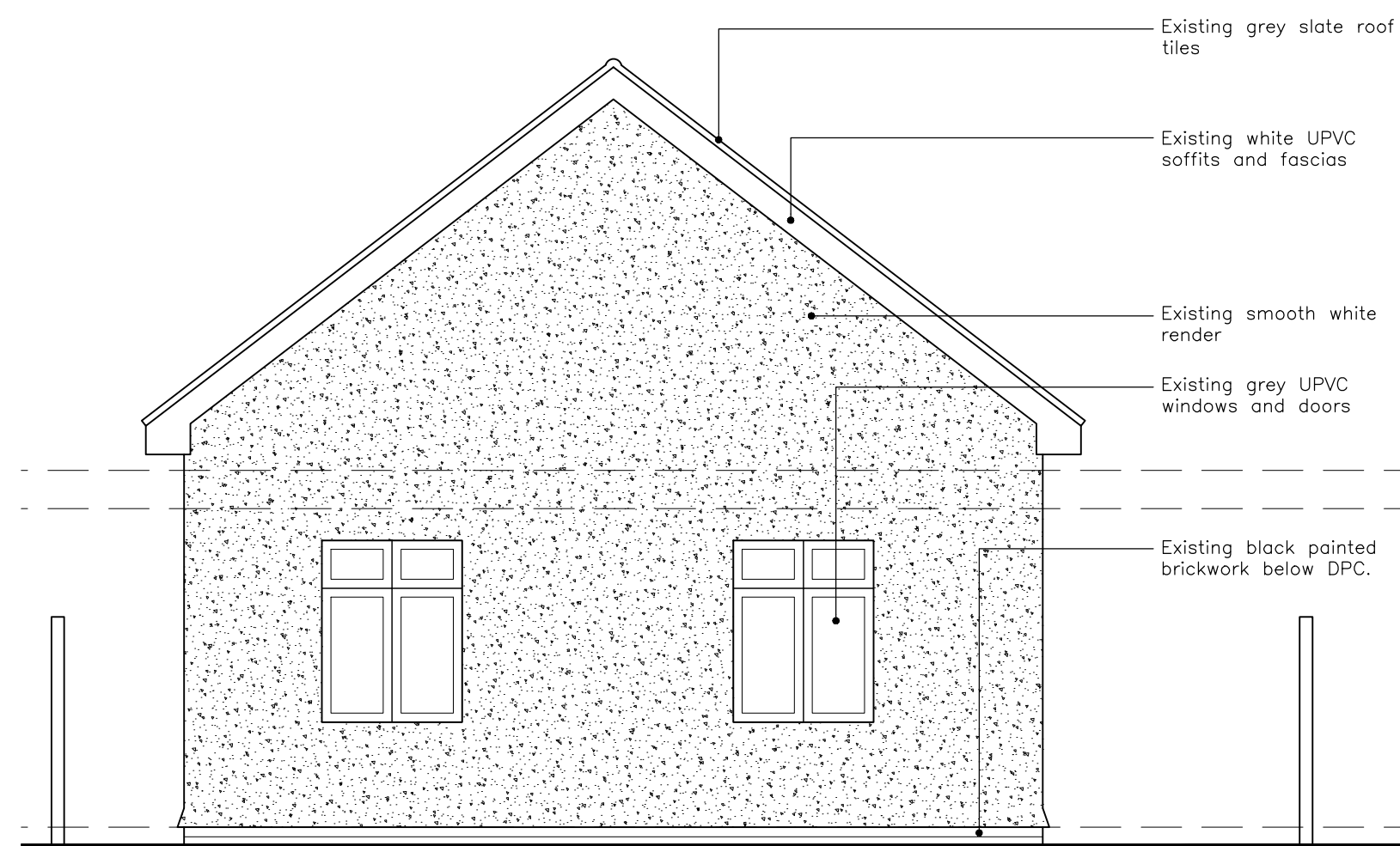
EXISTING FRONT ELEVATION 1:50@A1
