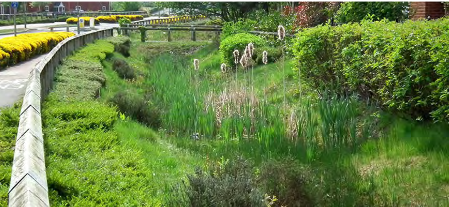
▲ The swales will be planted with suitable vegetation to create attractive landscape elements which benefit ecology and condition the surface water run-off
