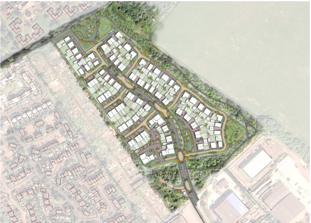
Revised design with raised tables providing visual and physical continuity of east-west routes.
