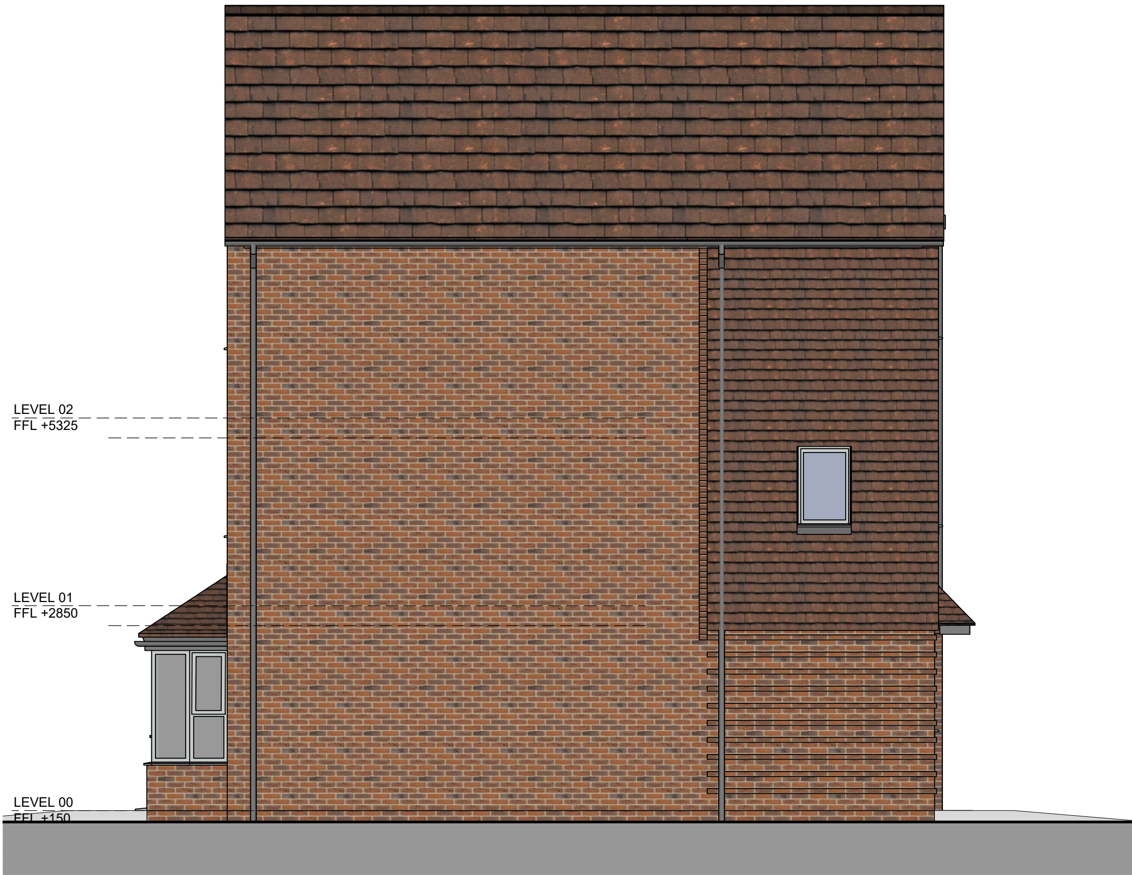
03 Side Elevation - Typical Scale 1:50 @ A1 (1:100 @ A3)
