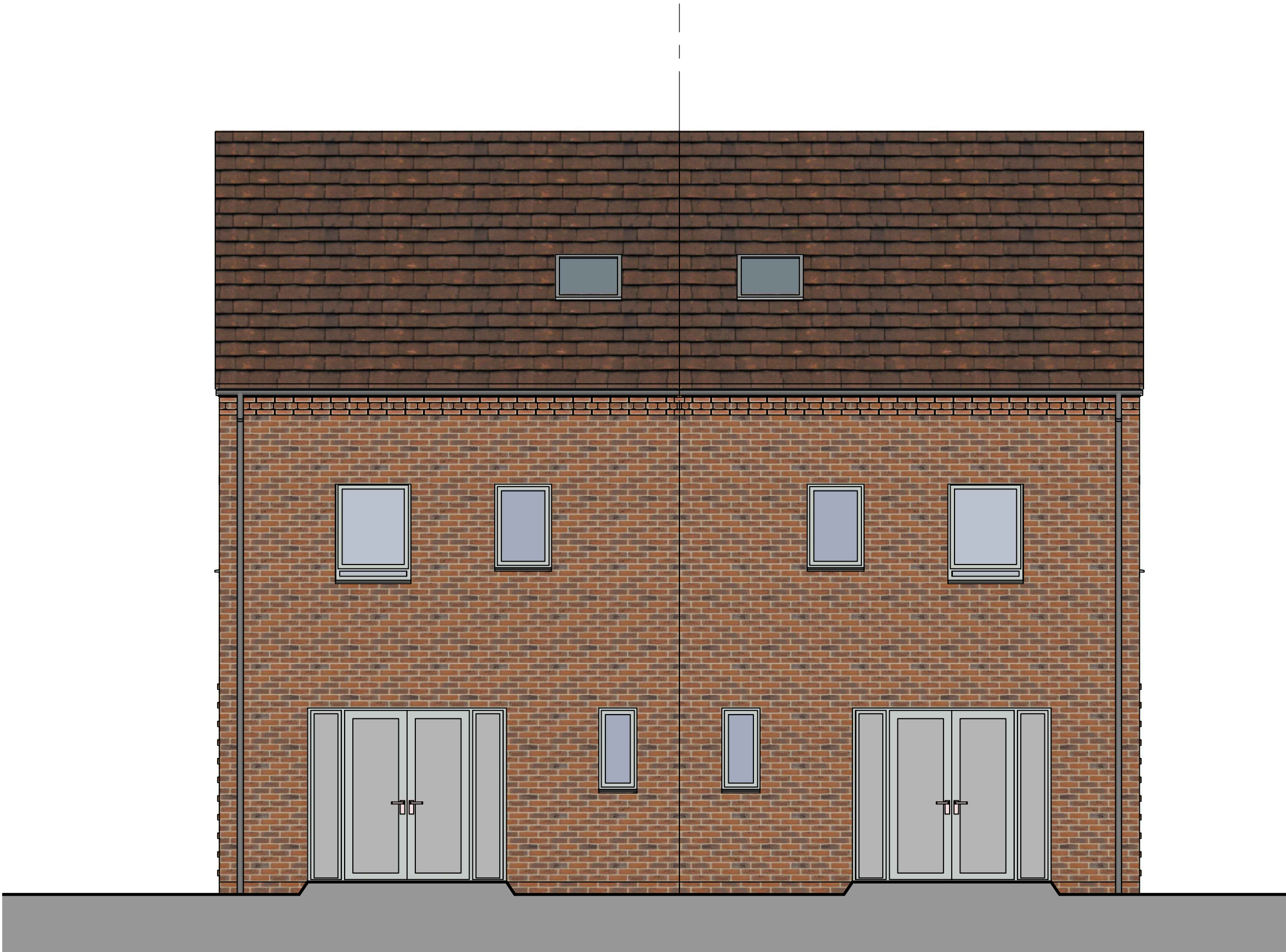
02 Rear Elevation - Typical Scale 1:50 @ A1 (1:100 @ A3)
