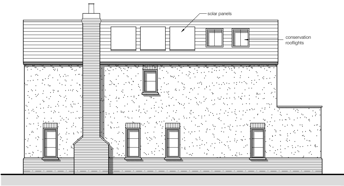
Side Elevation (south west facing)
