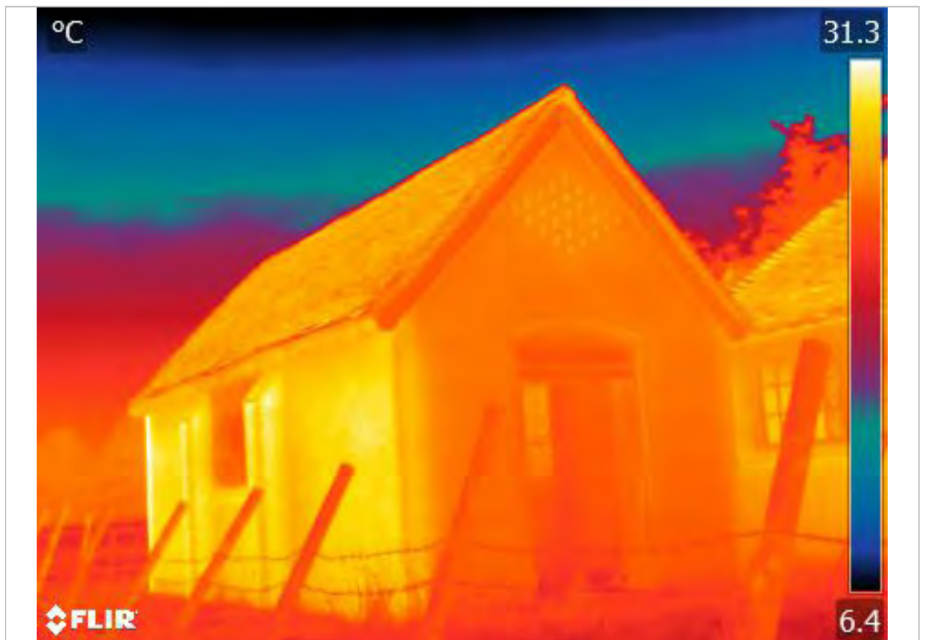
FLIR T860 (640 x 480 pixel resolution) with 42 degree lens = bat in flight detection distance of 66 m. Camera located 18 m from furthest point of building
