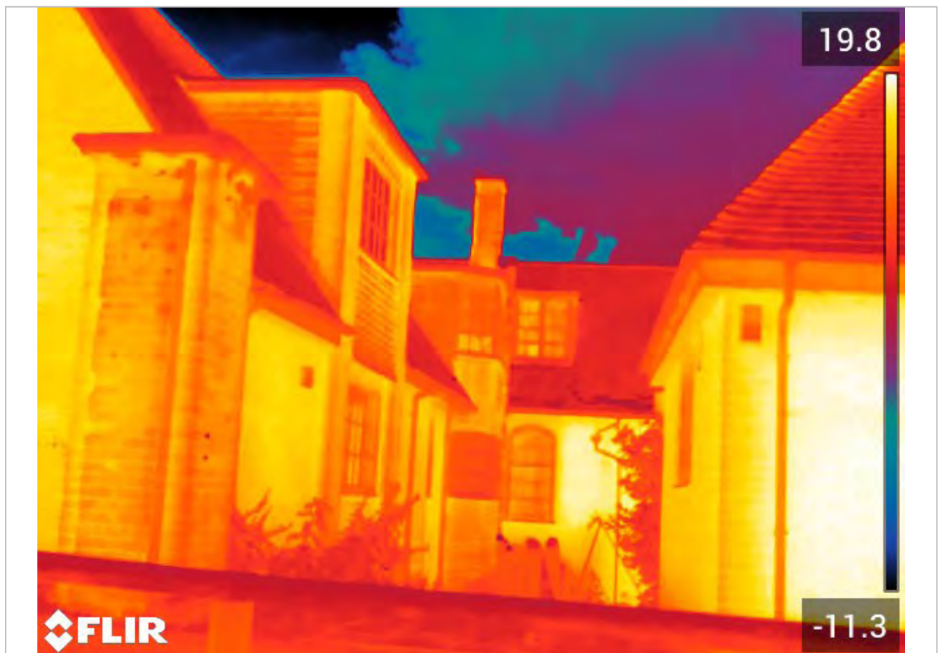
FLIR T540 (464 x 348 pixel resolution) with 42 degree lens = bat in flight detection distance of 51 m. Camera located 20 m from furthest point of building
