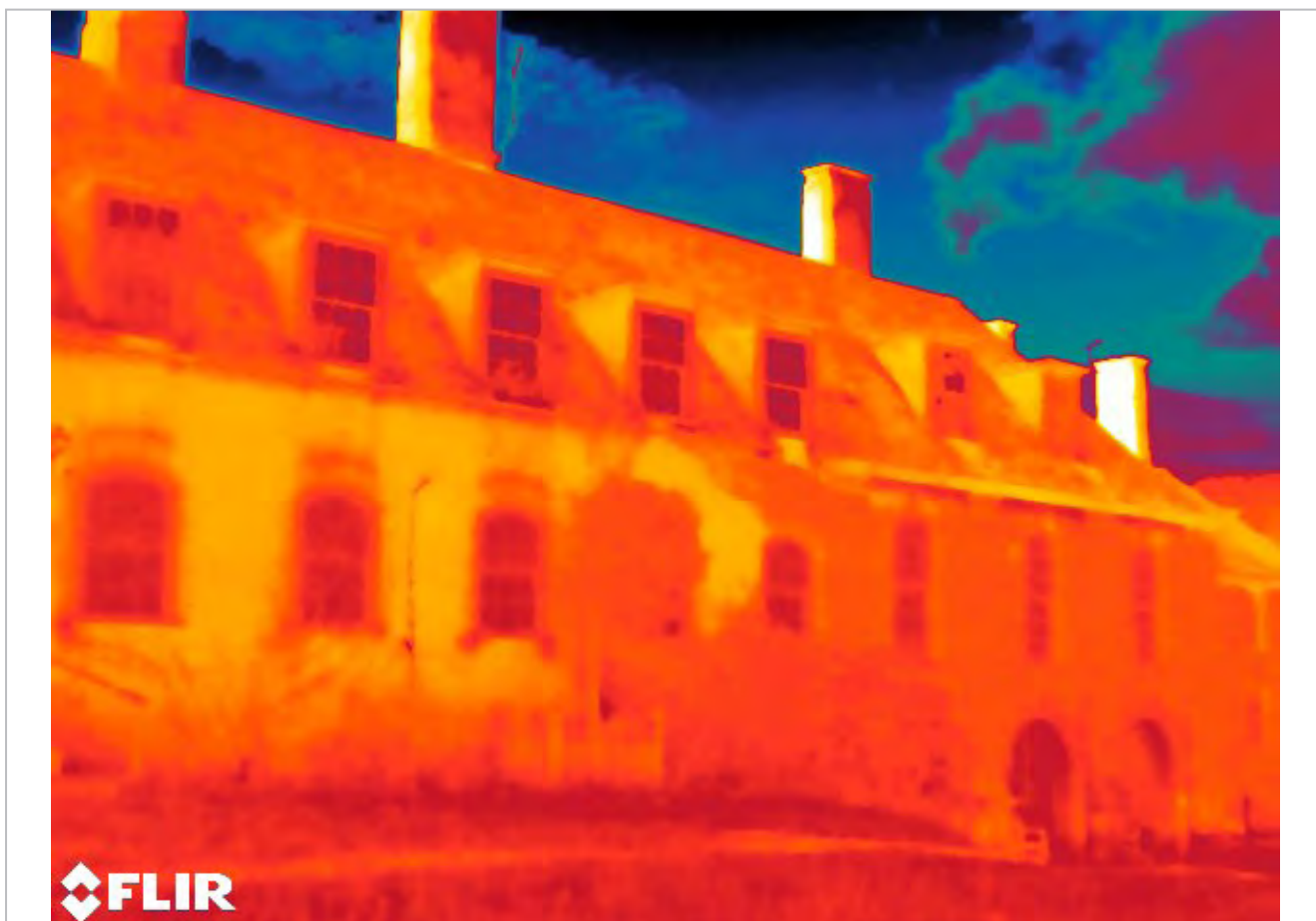
FLIR T860 (640 x 480 pixel resolution) with 42 degree lens = bat in flight detection distance of 66 m. Camera located 25 m from furthest point of building
