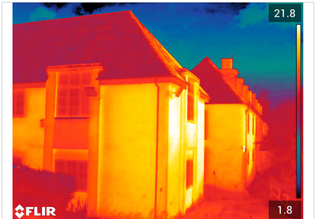
FLIR T1020 (1024 x 768 pixel resolution) with 45 degree lens = bat in flight detection distance of 104 m. Camera located 25m from furthest point of building
