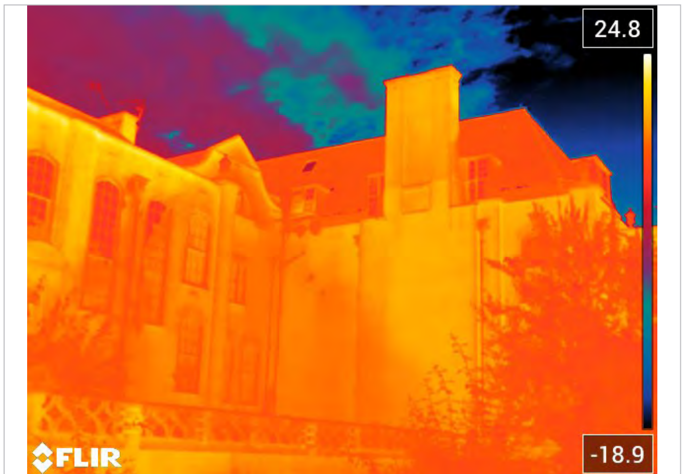
FLIR T540 (464 x 348 pixel resolution) with 42 degree lens = bat in flight detection distance of 51 m. Camera located 32 m from furthest point of building
