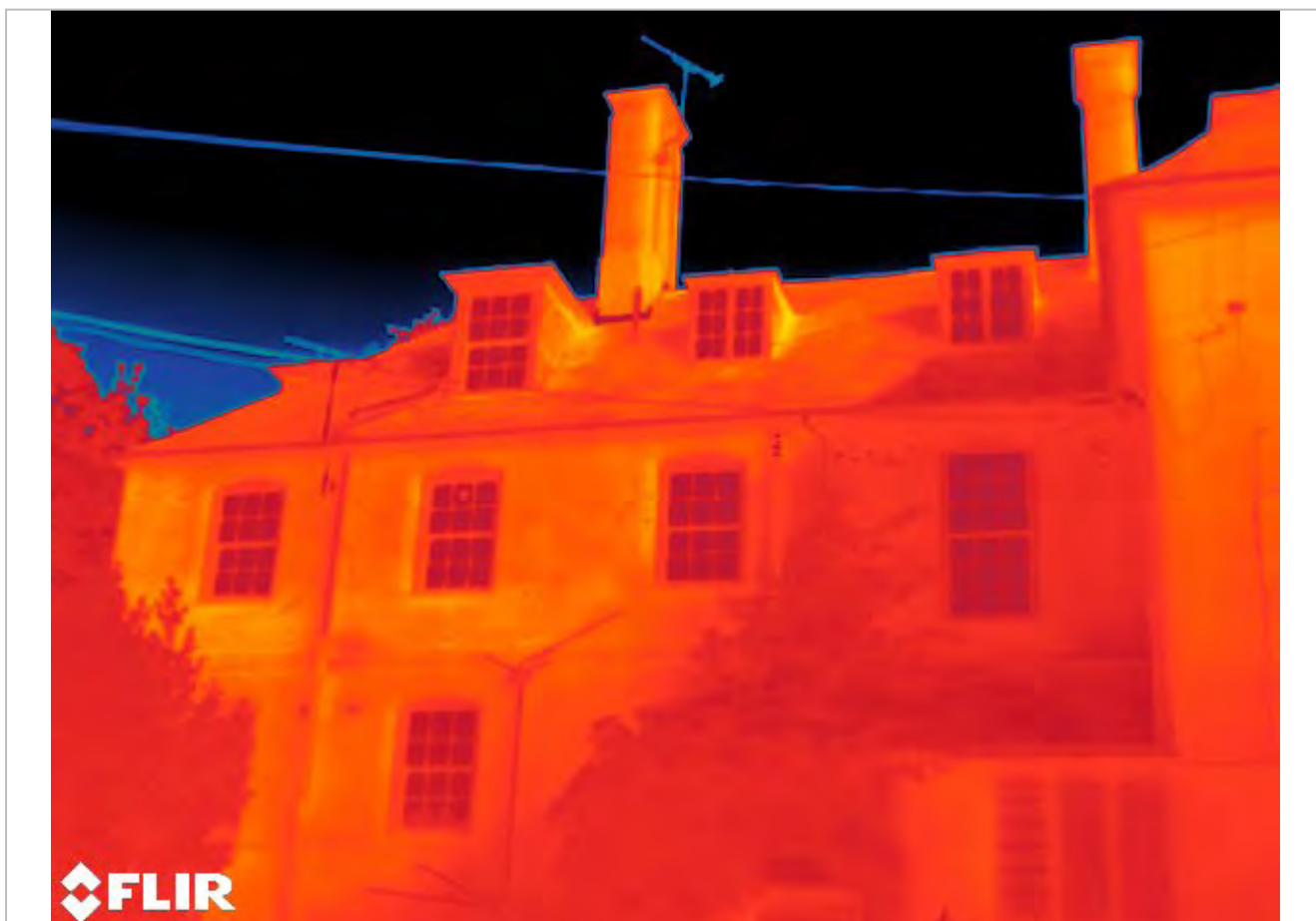
FLIR T540 (464 x 348 pixel resolution) with 42 degree lens = bat in flight detection distance of 51 m. Camera located 21 m from furthest point of building
