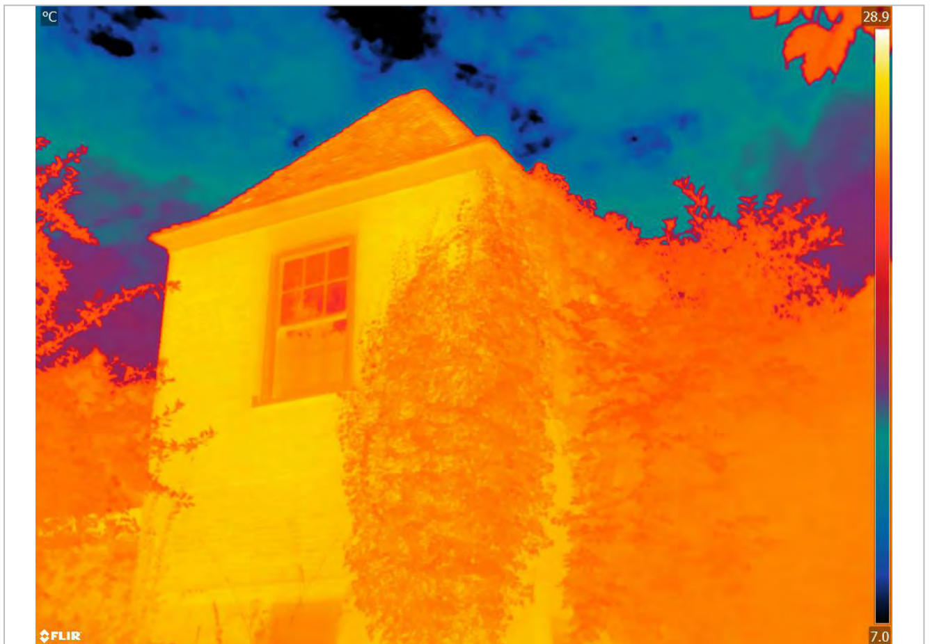
FLIR T1020 (1024 x 768 pixel resolution) with 45 degree lens = bat in flight detection distance of 104 m. Camera located 13 m from furthest point of building
