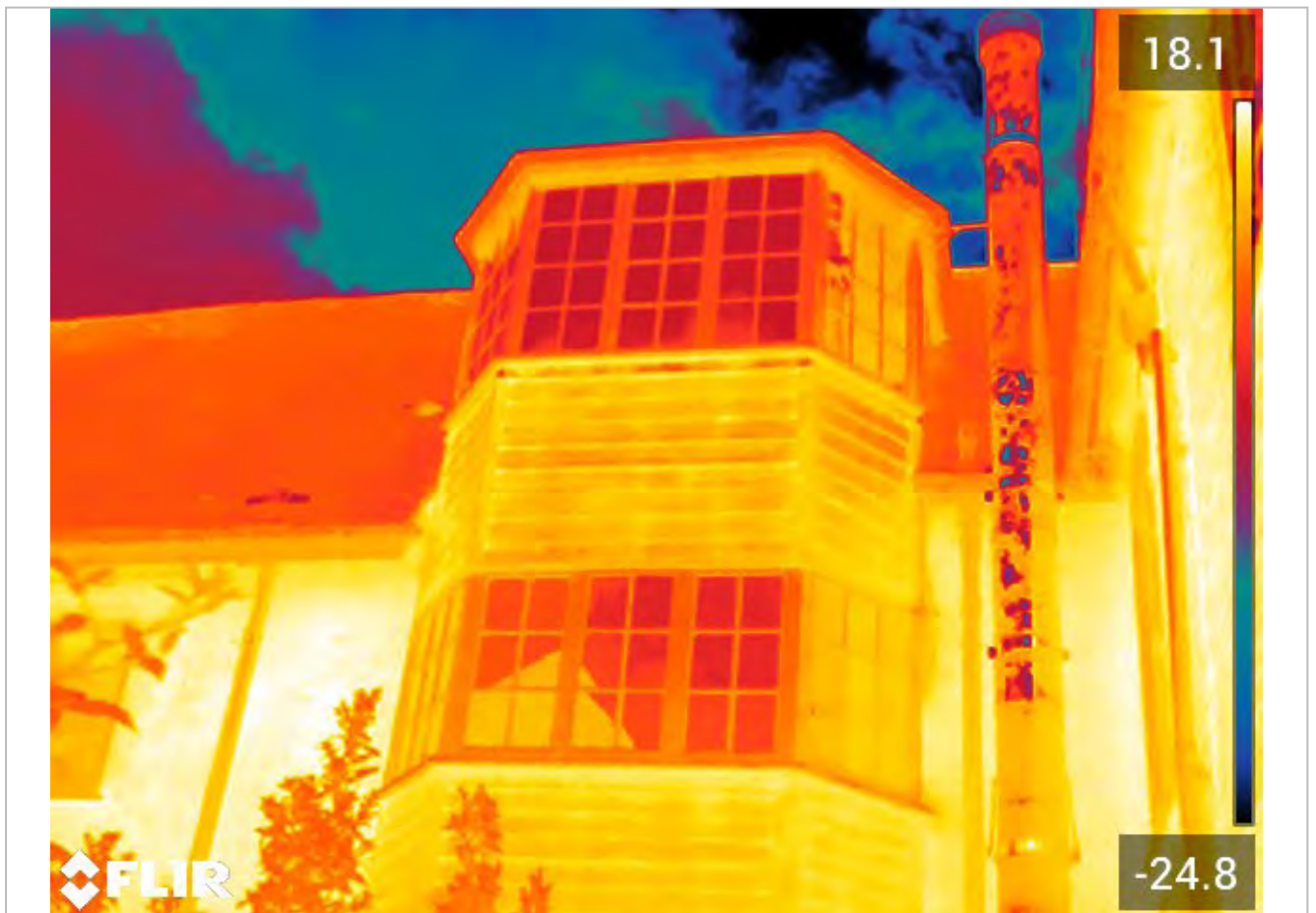
FLIR T540 (464 x 348 pixel resolution) with 42 degree lens = bat in flight detection distance of 51 m. Camera located 10 m from furthest point of building
