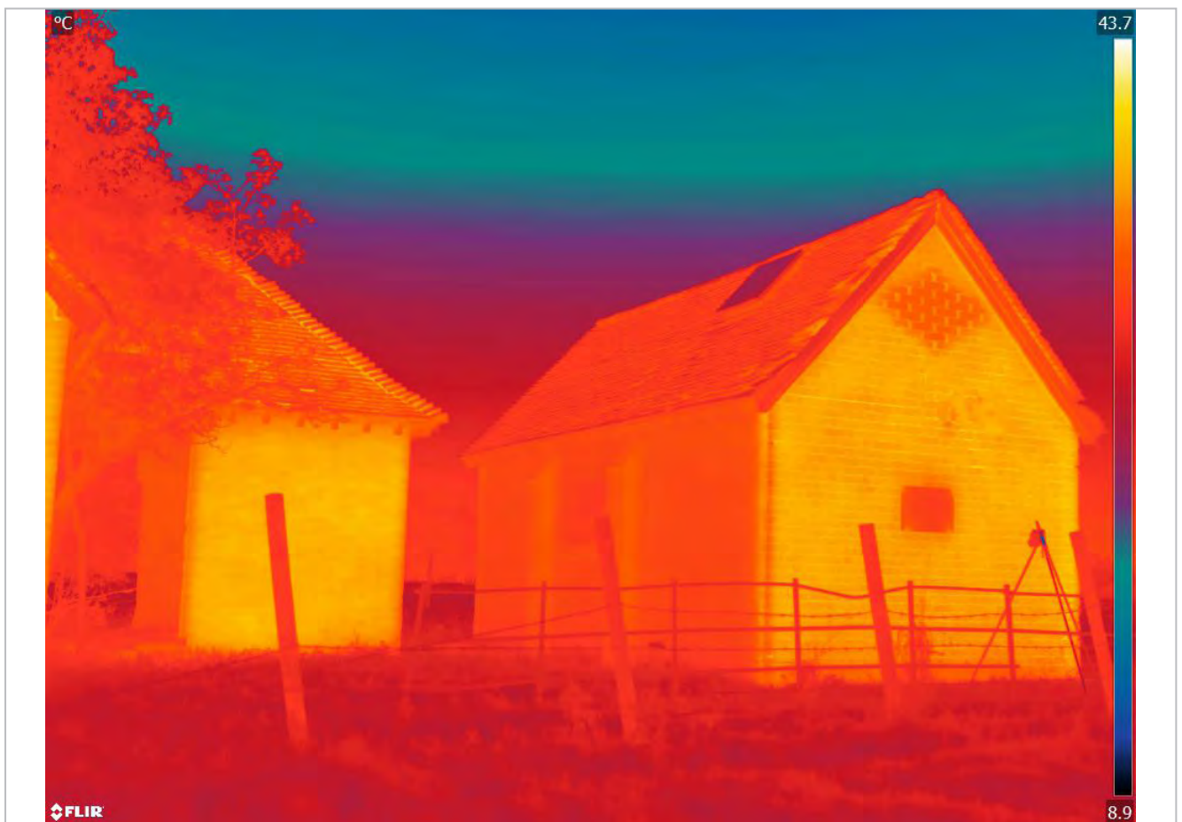
FLIR T1020 (1024 x 768 pixel resolution) with 45 degree lens = bat in flight detection distance of 104 m. Camera located 20 m from furthest point of building
