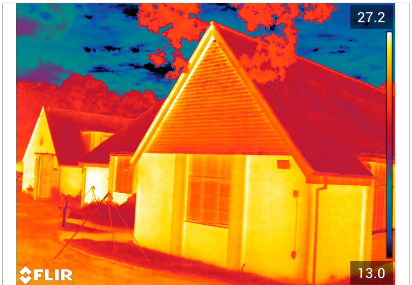
FLIR T1020 (1024 x 768 pixel resolution) with 45 degree lens = bat in flight detection distance of 104 m. Camera located 18 m from furthest point of building
