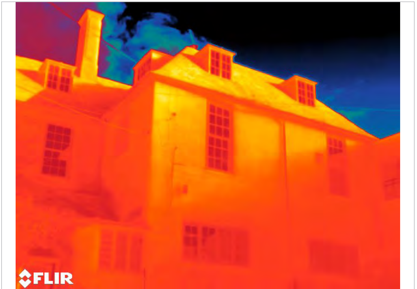
FLIR T540 (464 x 348 pixel resolution) with 42 degree lens = bat in flight detection distance of 51 m. Camera located 22 m from furthest point of building
