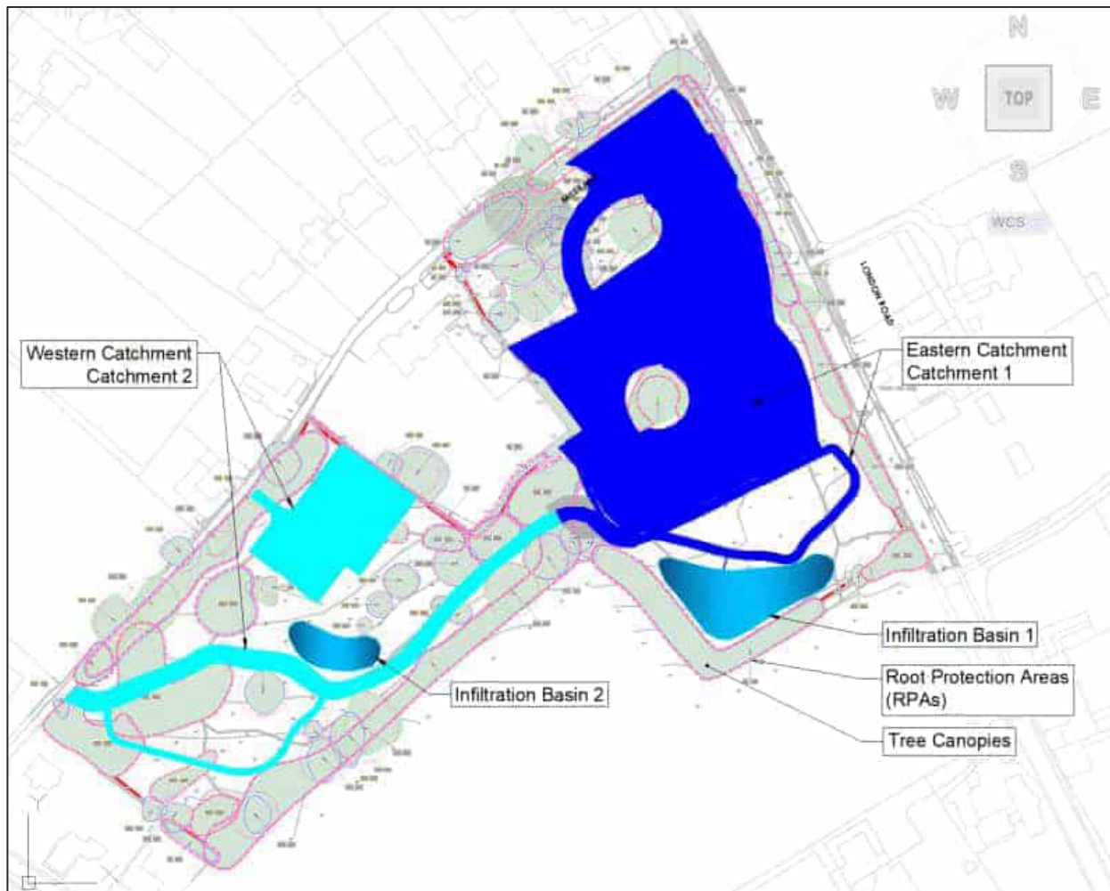
Figure 7-2 - Drainage Catchments and Infiltration Basins
