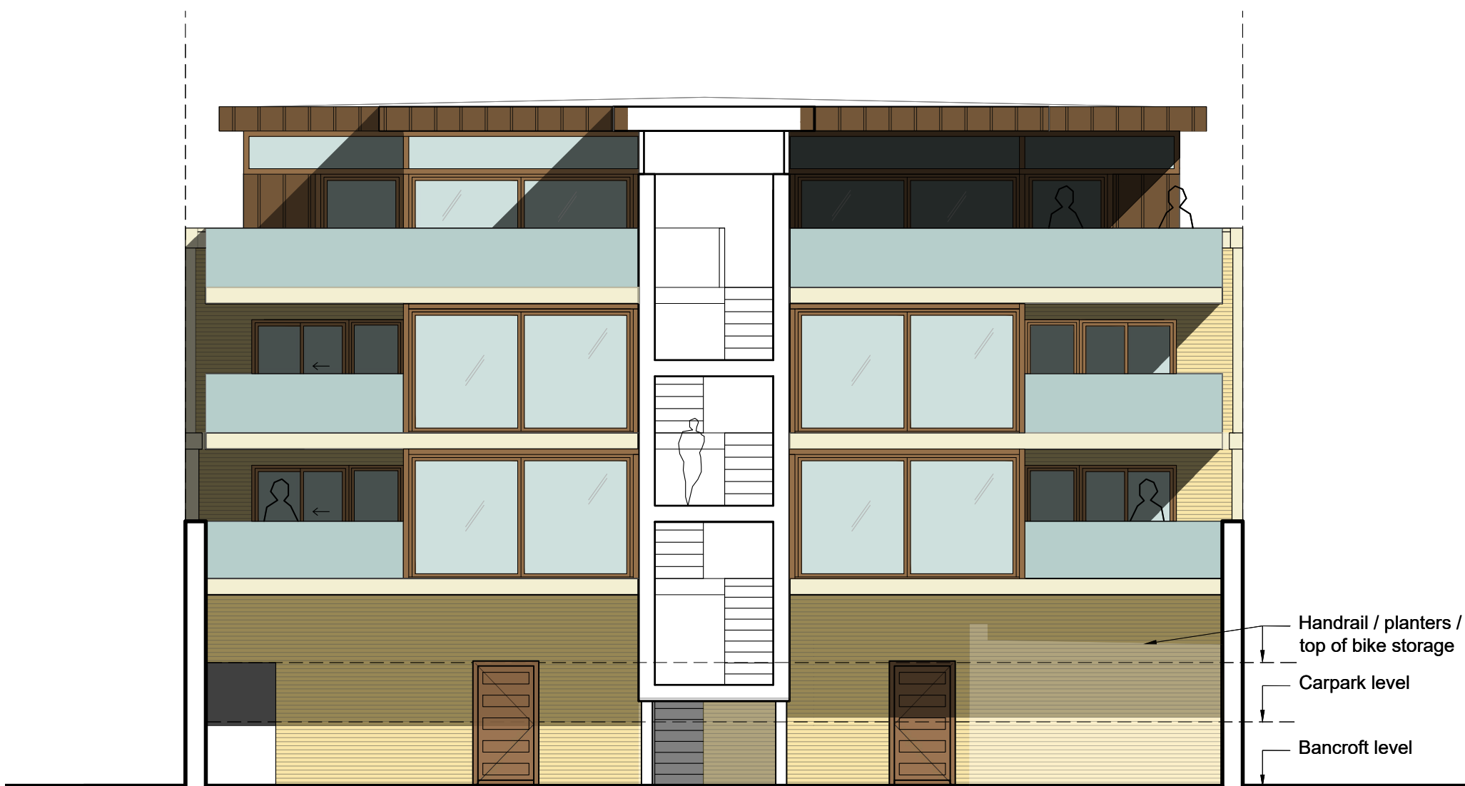
PROPOSED REAR ELEVATION & STAIR IN SECTION
