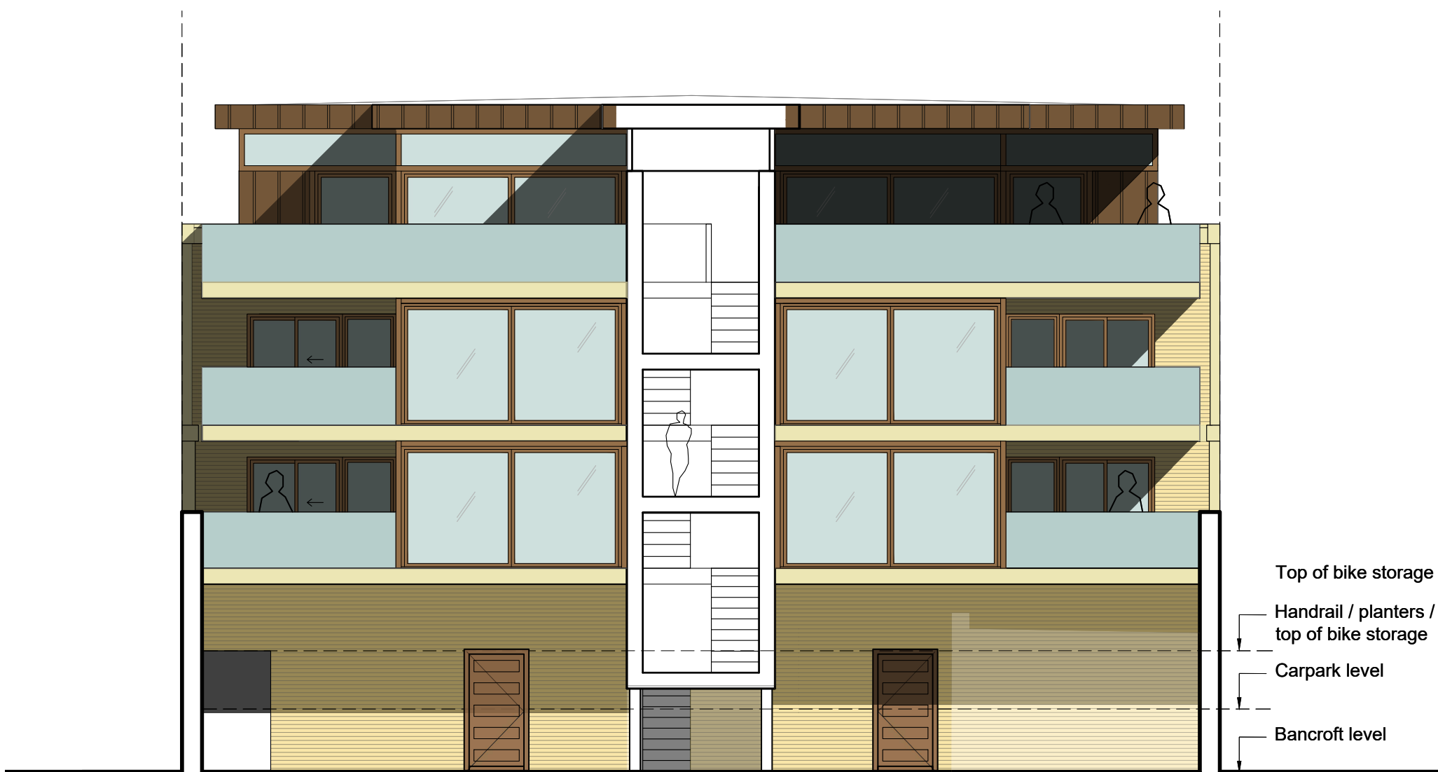
PROPOSED REAR ELEVATION & STAIR IN SECTION
