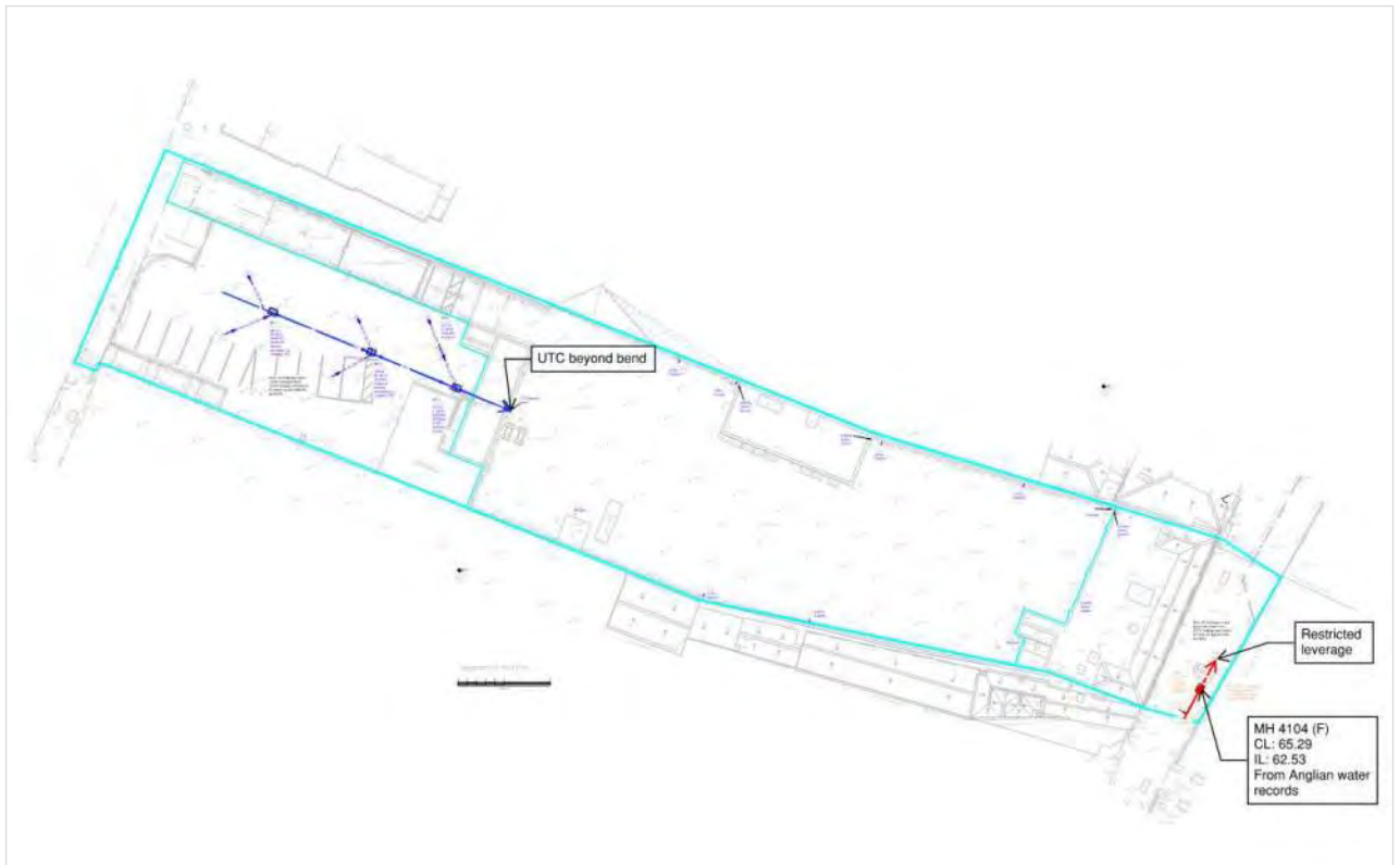
Figure 2.4: Drainage CCTV Survey Layout. (Source: Survey Solutions).
