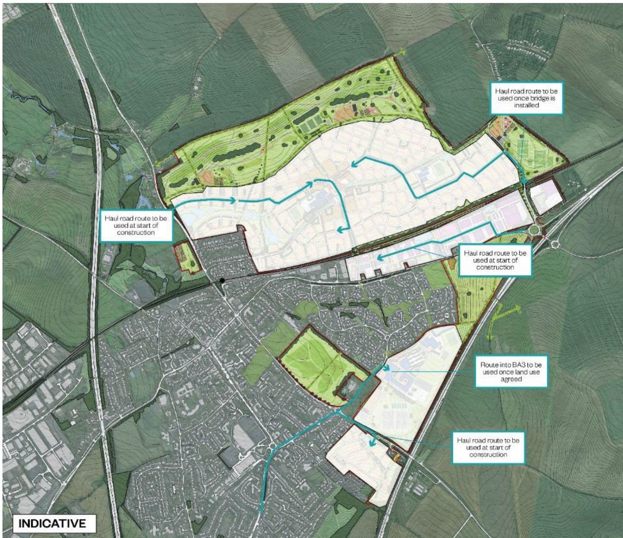
Figure 10-1: Proposed Outline Construction Routing Plan
