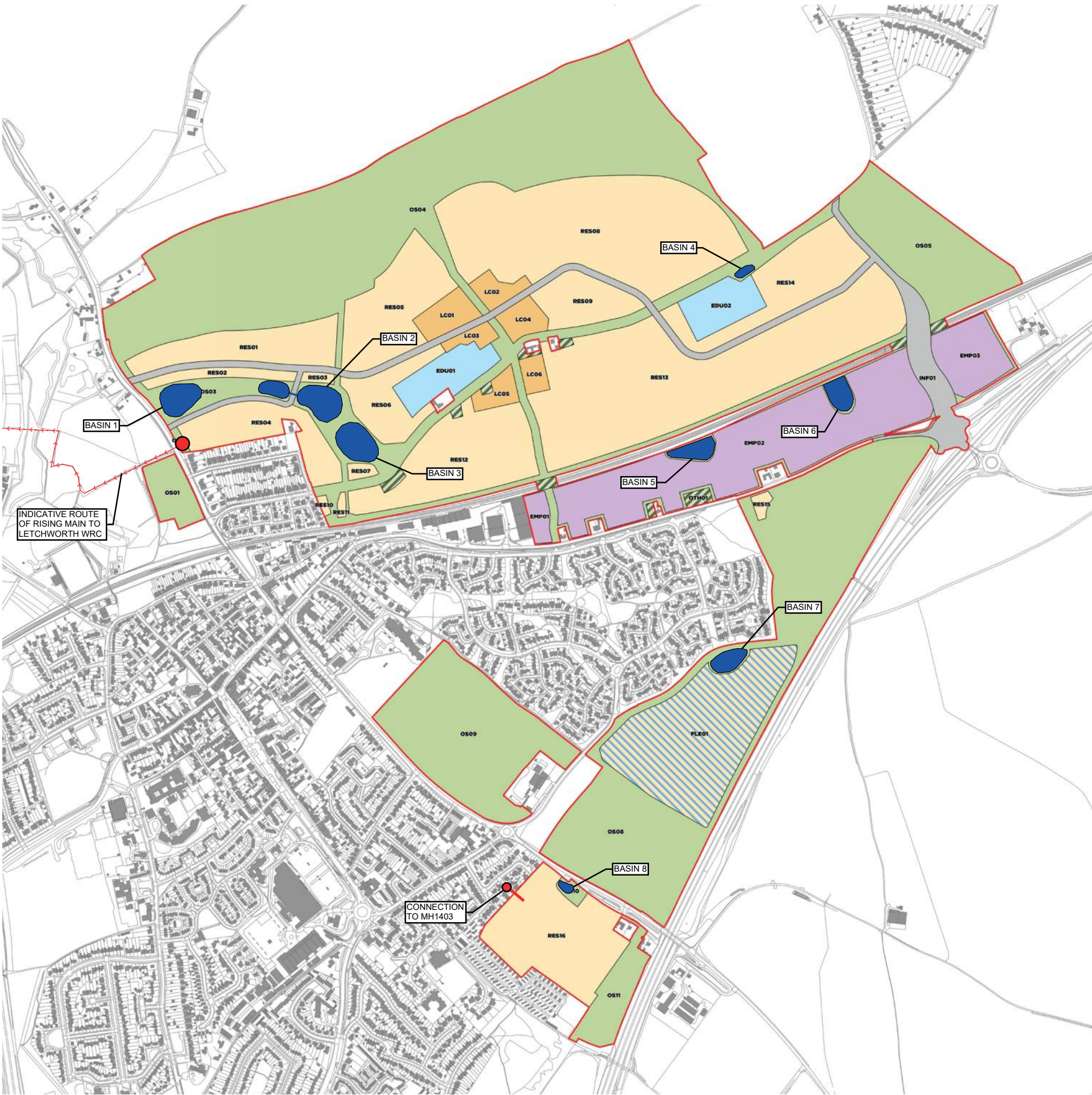
Figure 7.1 Infiltration basin and connection point locations
