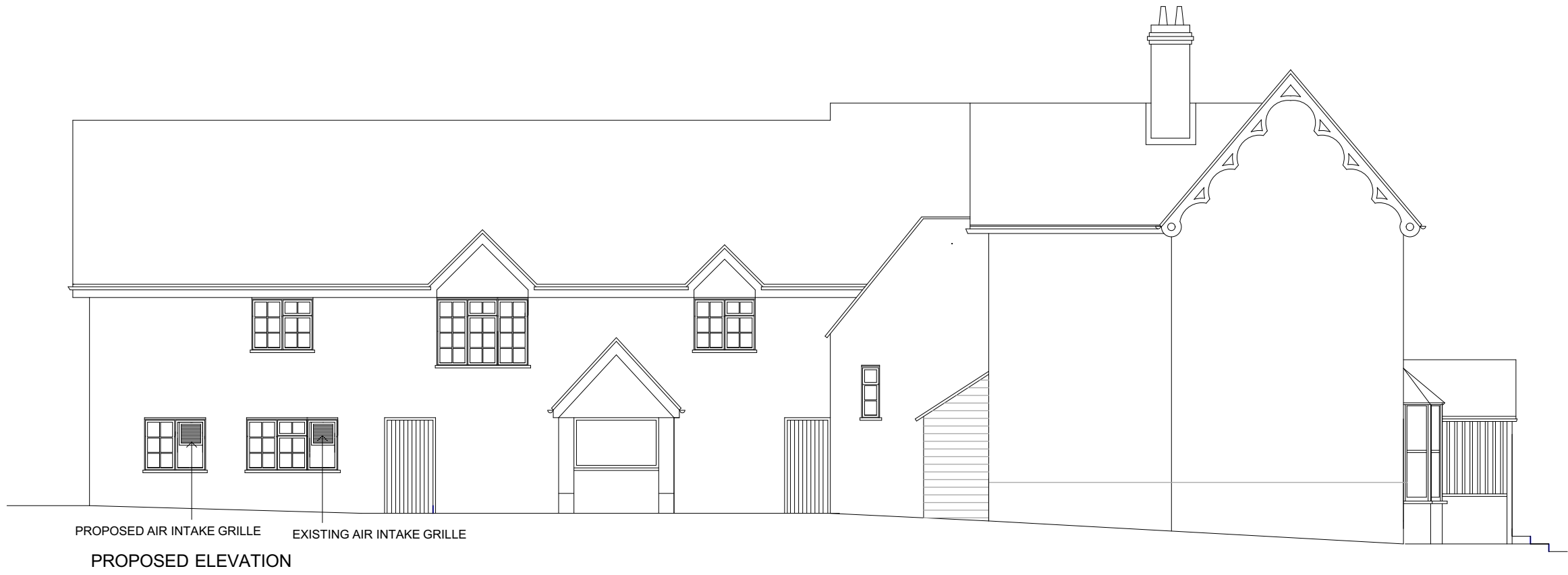
NEW AIR INTAKE GRILLE - 500MM X 500MM METAL CASING INTERNAL PLATE AXIAL FAN AS ABOVE
