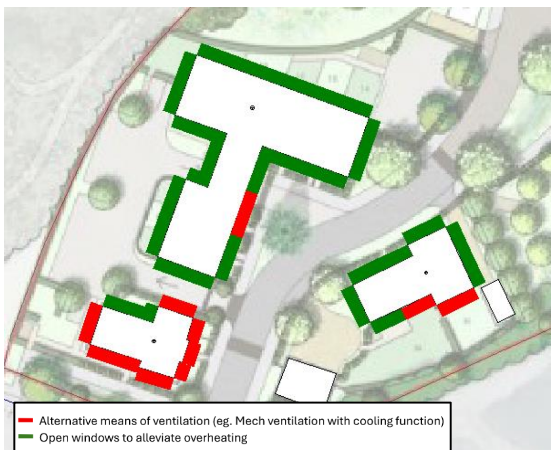
Figure 7.1: Overheating assessment and ventilation – Plots 1-4, 5-14 and 37-38
