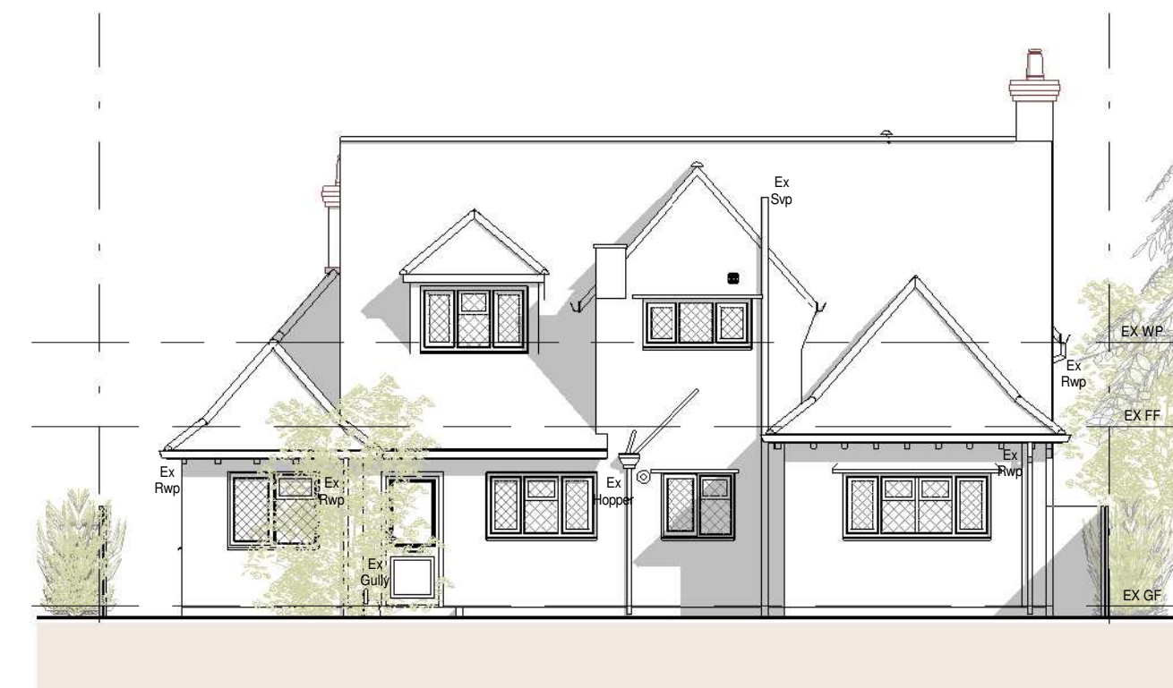
5 Existing North Elevation 1 : 100
