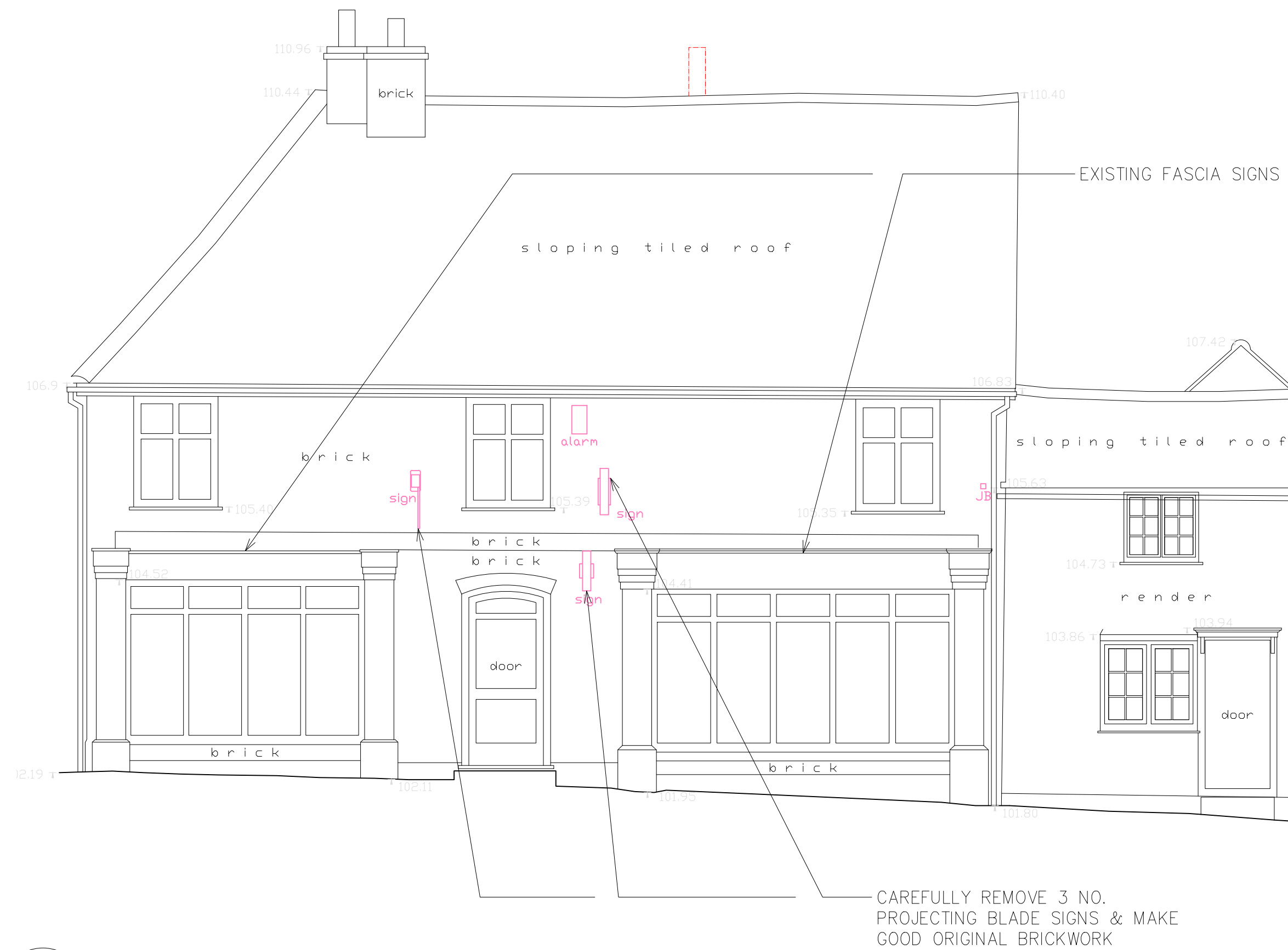
1 EXISTING FRONT ELEVATION 1 : 50
