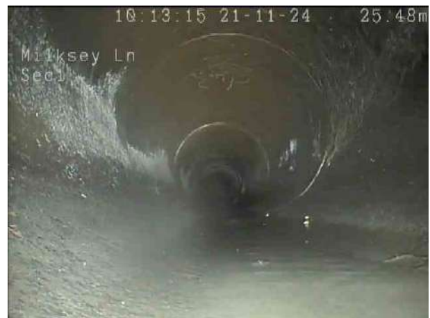
7b70e5a9-b297-4289-a504-2282be5e6a94.png, 00:01:30, 25.50 m Roots, fine at joint, finish
