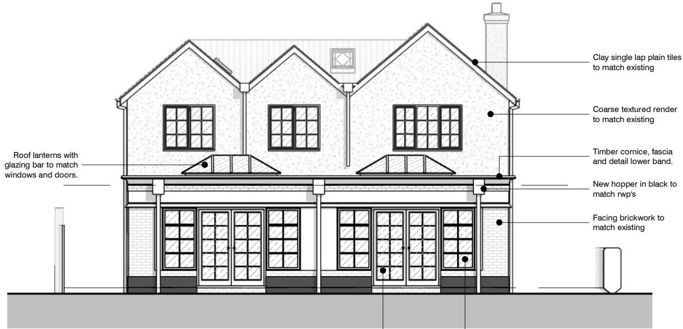
3 Rear Elevation - PROPOSED - B 1 : 100 @A3
