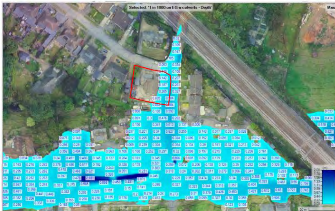
Figure 5.47: Flood Inundation Map – Depth (1:1000 year, with culverts)
