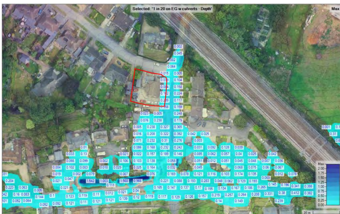
Figure 5.2: Flood Inundation Map – Depth (1:20 year, with culverts)
