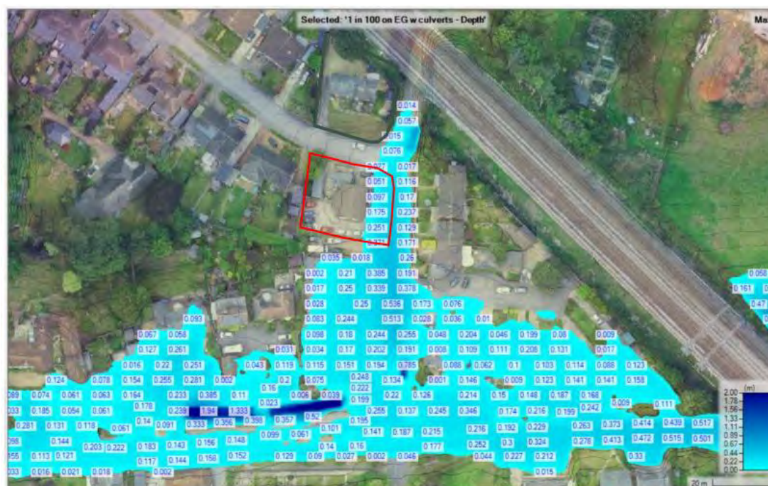
Figure 5.21: Flood Inundation Map – Depth (1:100 year, with culverts)
