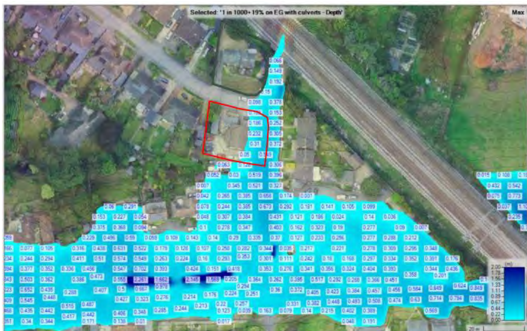
Figure 5.53: Flood Inundation Map – Depth (1:1000+19% year, with culverts)
