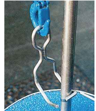
Step 3 – Lower the 'lifting hook' down the shaft to the bottom bracket.
