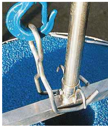
Step 5 – Once passed the lifting hooks, swivel the 'lifting hook' through 90° to allow it to saddle the bottom bracket and position itself under the lifting hooks.
