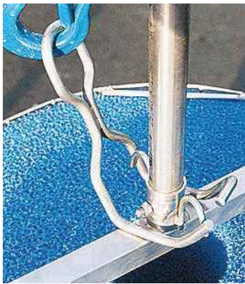
Step 4 – Swivel the hoist chain until the 'lifting hook' is at 90° to the bottom bracket, allowing it to pass the lifting hooks welded each side of the bottom bracket.
