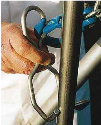
Step 1&2 – Snap the 'lifting hook' onto the SPEL lifting/locating/locking system handle shaft.
