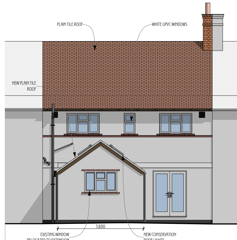
E-02 North West Elevation 1:100
