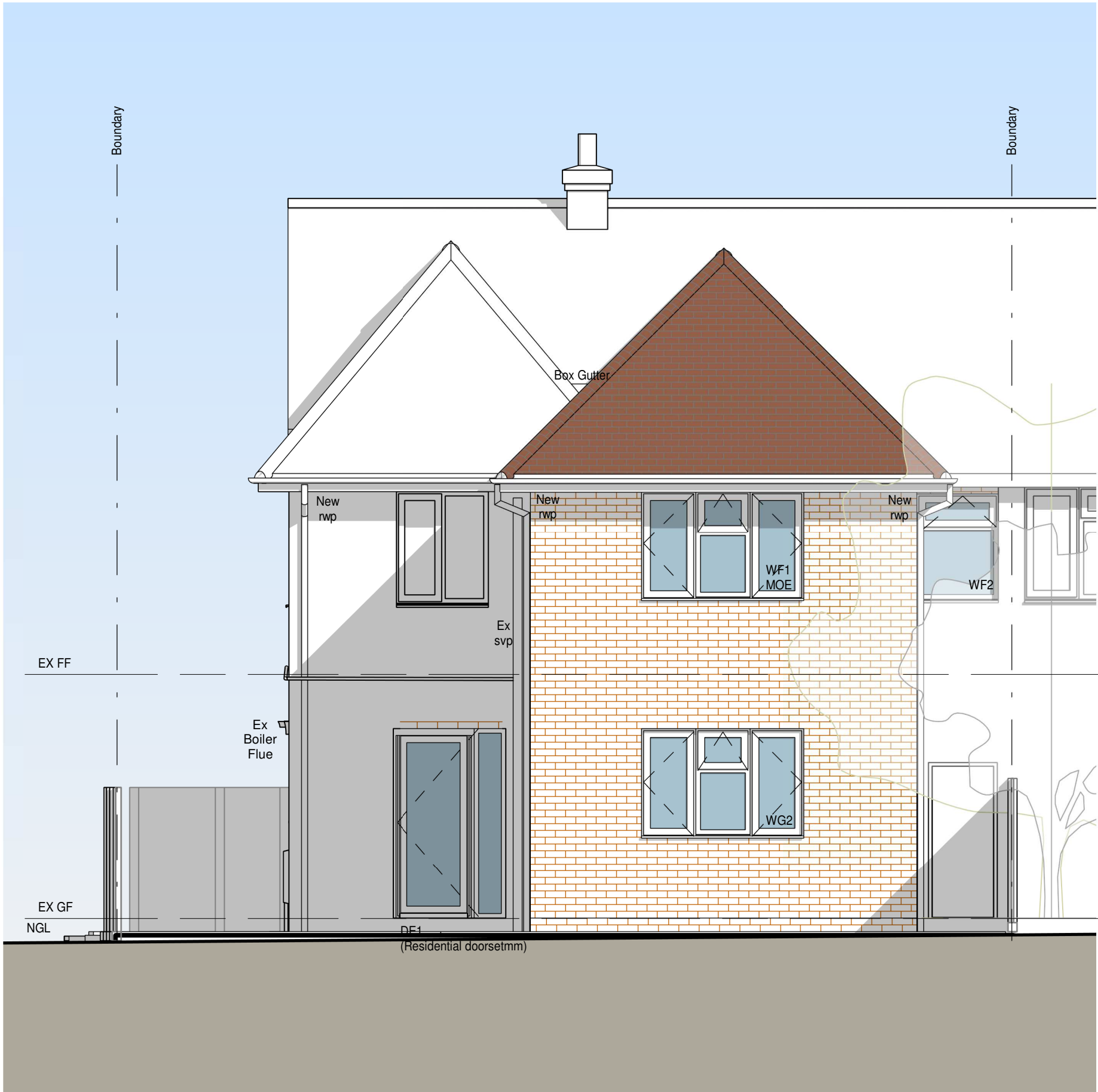
2 Proposed South West Elevation 1 : 50
